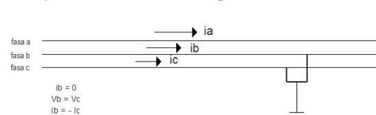
Fig 3. Two-phase short circuit to ground
