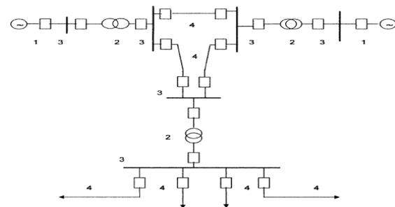
Fig 6. One line diagram of an electric power system with its safety zones
