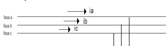
Fig 4. 3-phase short circuit fault
