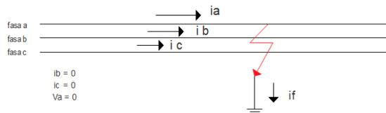
Fig 1. Single phase short circuit to ground
