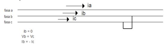
Fig 2. Two-phase short circuit Gangguan
