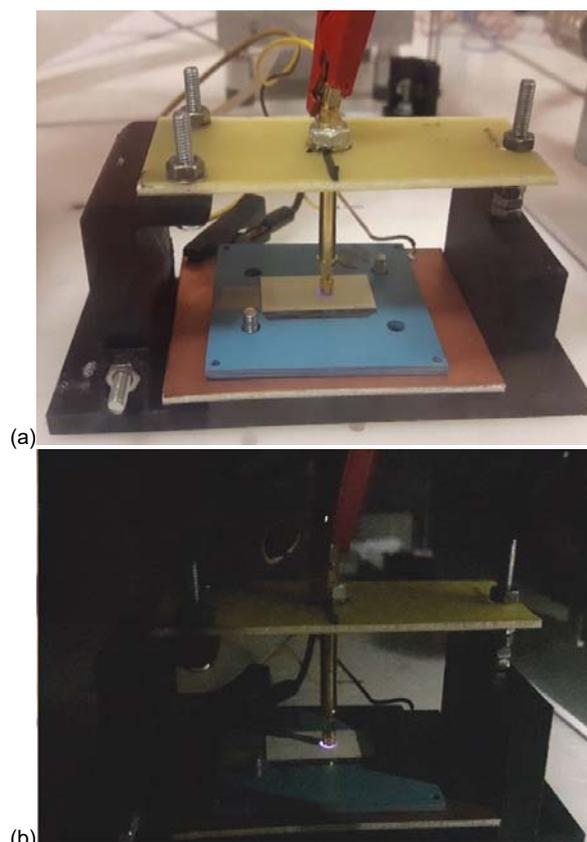
Fig.4. Stand for plasma surface modification before operation (a) and during modification (b)
