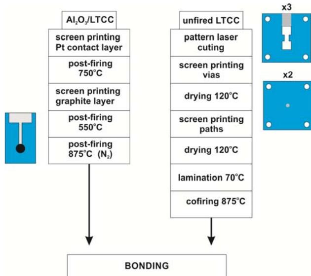
Fig.2. Technology of preparing structures for bonding tests
