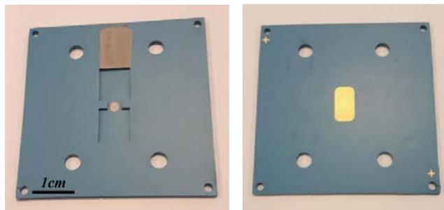
Fig.3. LTCC part with cofired metallizations: top side – bonded side (a) and bottom side (b).
