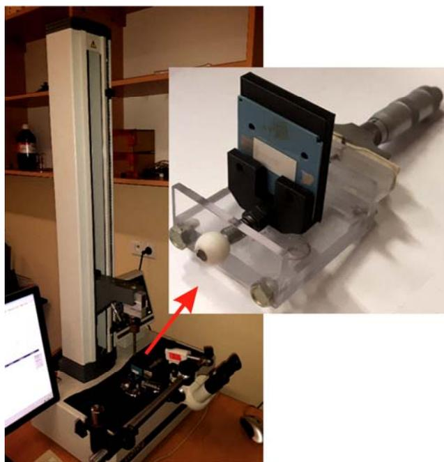
Fig.5. Machine testing the strength of the connection with the zoom of the sample fixing
