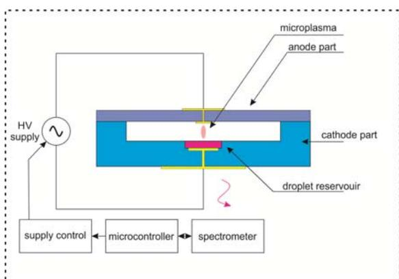
Fig.1. Schematic operation of sensor based on microplasma generator
