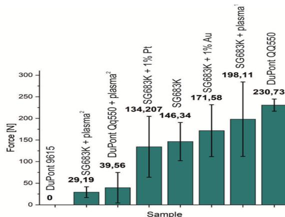
Fig.6. Average value of the forces obtained for individual methods of joining with their standard deviation (<sup>1, 2</sup> plasma modification of the surface for 5 and 10 minutes, respectively)
