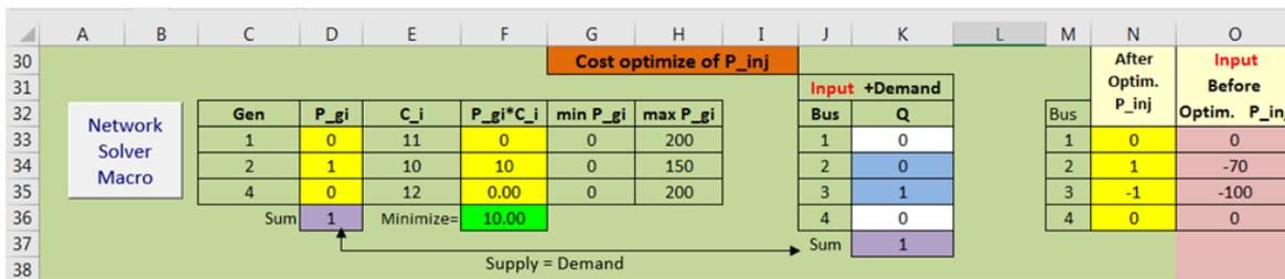
Fig.3. Economic dispatch solver for  $S_{M,23}$  with button 'Network Solver Macro' activate the solver
