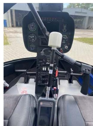
Fig.1 Reference drawing of electric field measurement with a meter with 01E measuring probe in Robinson R44 Raven helicopter.
