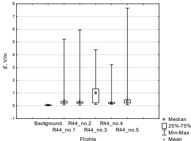
Fig.3 Box plots of measurement of electric component of electromagnetic fields
