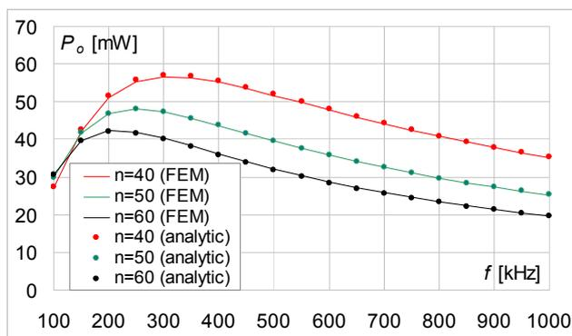
Fig.8. Results comparison of receiver power ( $P_o$ ) dependent of number of turns for the case  $h = 25$  mm
