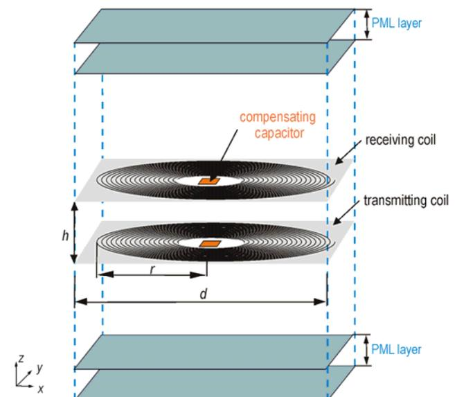
Fig.2. A three-dimensional view on one of WPT cell
