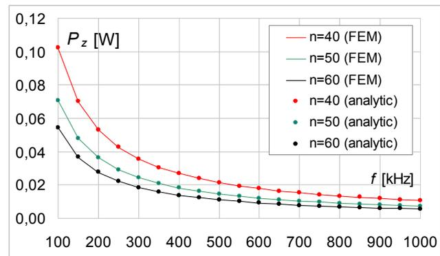
Fig.4. Results comparison of source power ( $P_z$ ) dependent of number of turns for the case  $h = 12.5 \text{ mm}$
