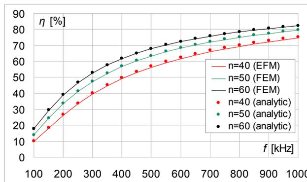
Fig.9. Results comparison of power transfer efficiency dependent of number of turns for the case  $h = 25$  mm
