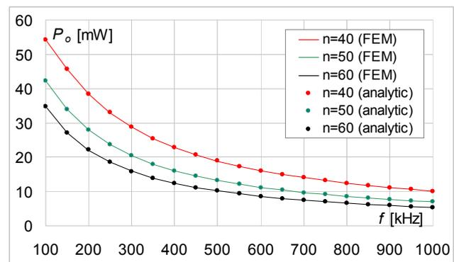
Fig.5. Results comparison of receiver power ( $P_o$ ) dependent of number of turns for the case  $h = 12.5 \text{ mm}$
