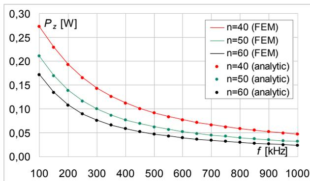
Fig.7. Results comparison of source power ( $P_z$ ) dependent of number of turns for the case  $h = 25$  mm
