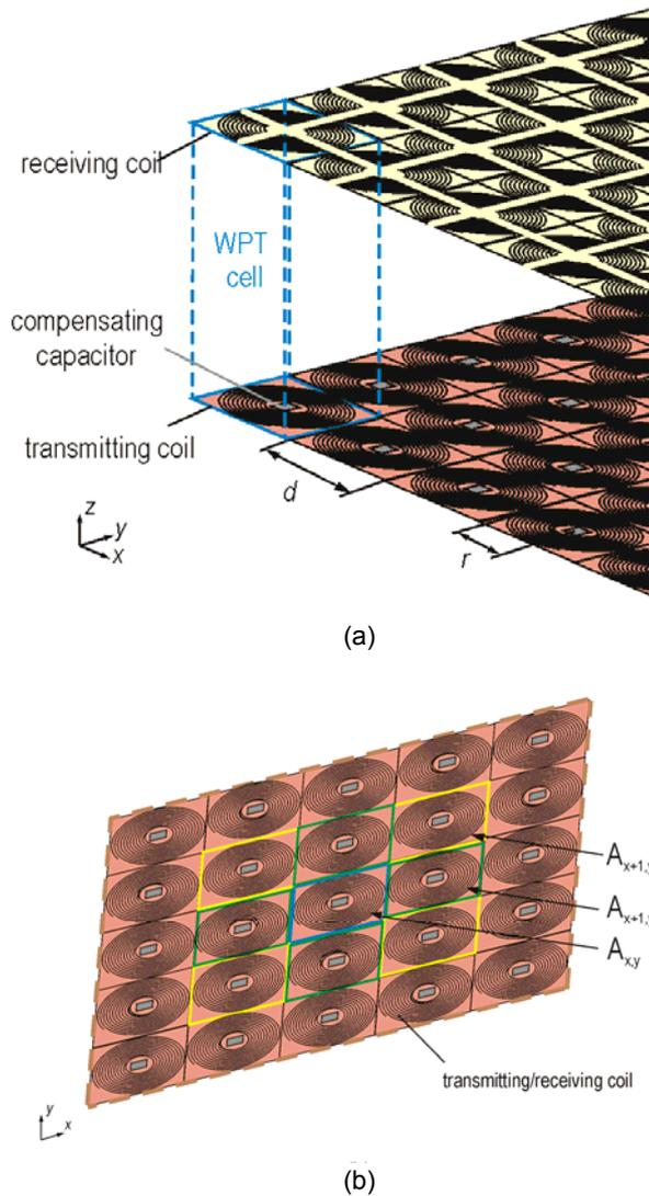
Fig.1. WPT system: (a) periodic wireless power transfer system composed of transmitting surface (bottom) and receiving surface (on top), (b) a fragment of the transmitting/receiving surface
