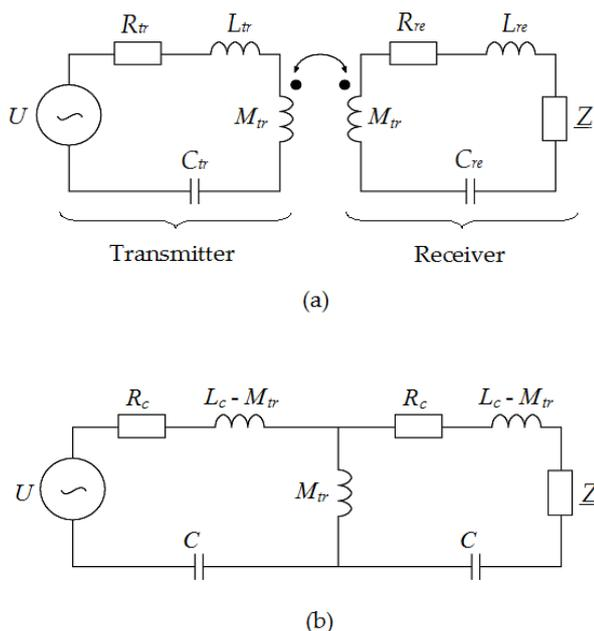
Fig.3. Analytical model of the periodic WPT cell: (a) overall model of periodic cell, (b) replacement model of the cell for identical transmitting and receiving coil
