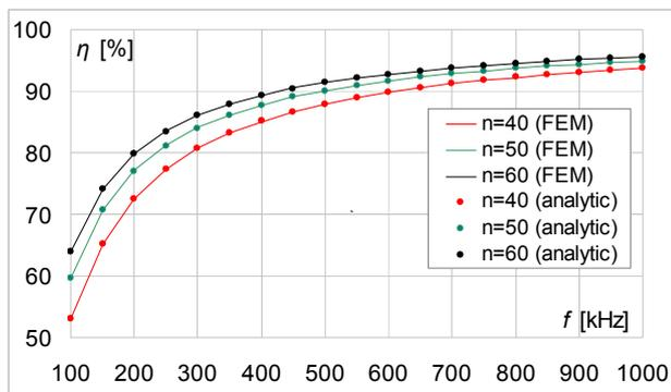
Fig.6. Results comparison of power transfer efficiency dependent of number of turns for the case  $h = 12.5$  mm
