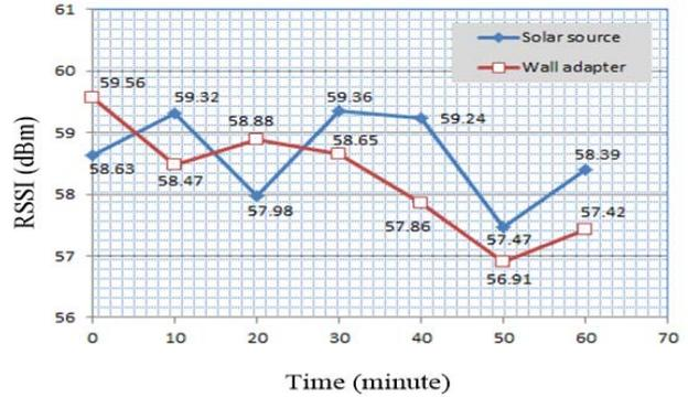
Fig. 6 The measured RSSI values at different test times
