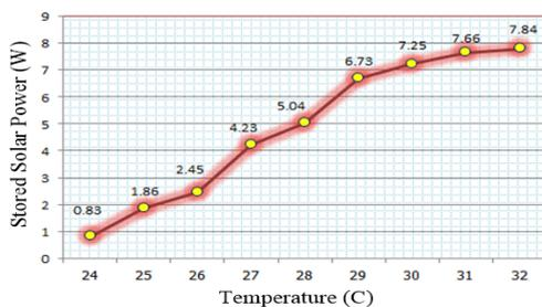
Fig. 3 The storage of solar's power according to temperature variable
