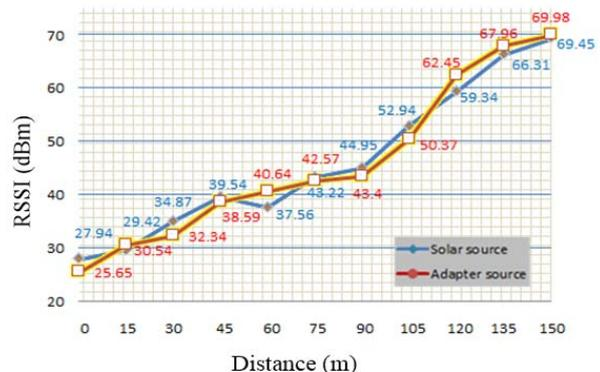
Fig.7 Comparison of the measured RSSI from solar source and adapter
