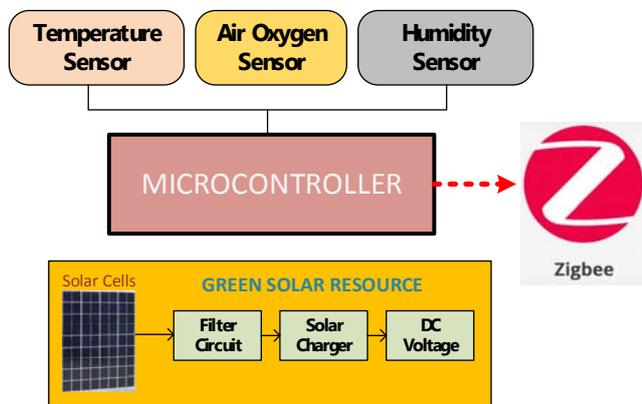
Fig. 1 Block diagram of wireless environment monitoring supplied by the green solar resource
