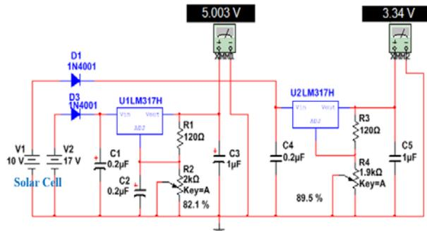
Fig. 2 Solar charger schematic circuit
