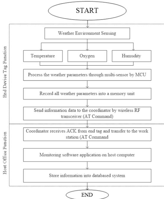
Fig. 5 Data flow process of the end tags and the coordinator
