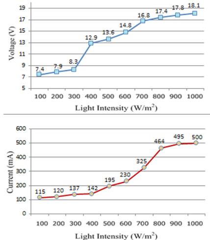
Fig. 4 The production of voltage and current according to light intensity
