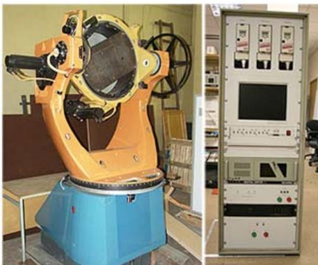
Fig. 3. Three-degree semi-natural modeling stand
