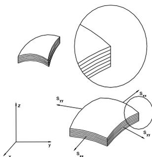
Fig.1. Multilayer three-four-angle shell finite element
