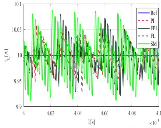
Fig.12. Output current ripple of Buck converter with each controllers in steady state
