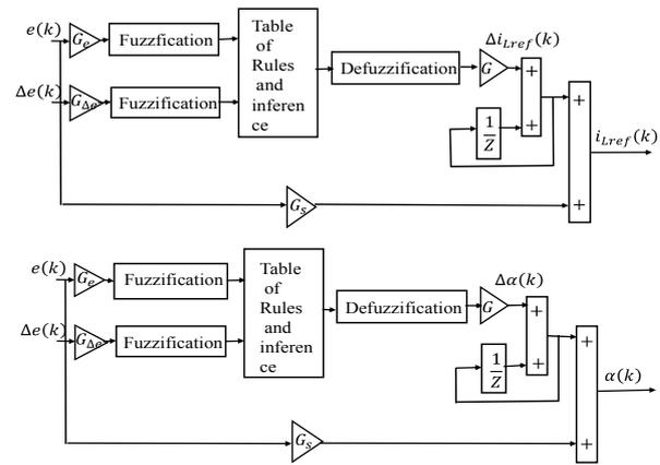
Fig.4. Model of fuzzy logic controller for output voltage and current Figure 5 represents the membership functions for the error, change in error, and the output [9, 18].
