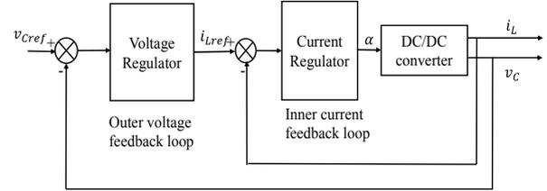
Fig.2. Proposed PI controller for Buck chopper
