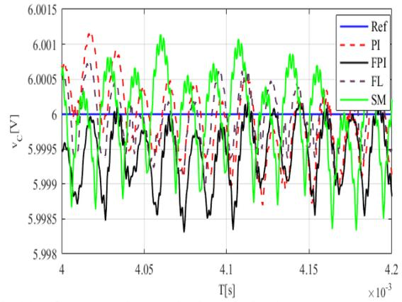
Fig.11. Output voltage ripple of Buck converter with each controllers in steady state
