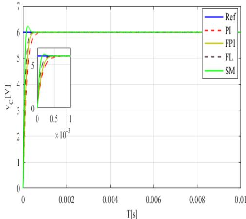
Fig.8. Output voltage of parallel multicellular Buck converter with the four controllers
