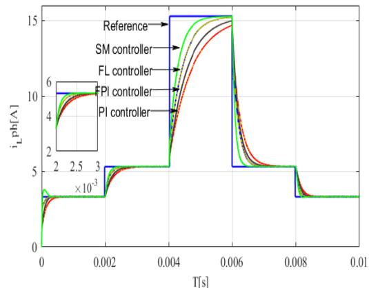
Fig.17. Dynamic responses of phases current with changes in load using the controllers
