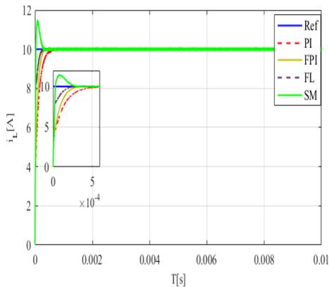
Fig.9. Output current of parallel multicellular Buck converter with the four controllers
