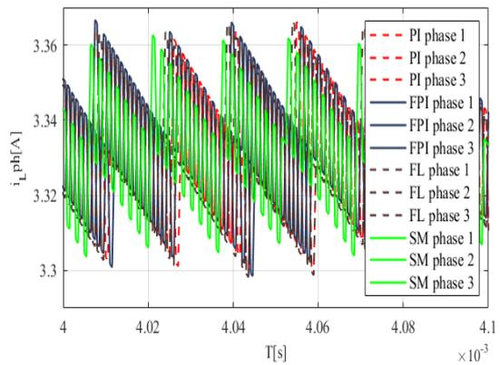
Fig.13. Phases current ripple of Buck converter with each controllers in steady state
