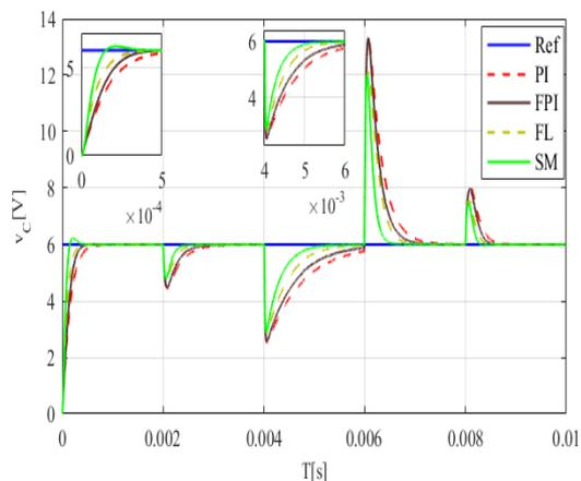
Fig.15. Dynamic responses of output voltage with changes in load using the controllers
