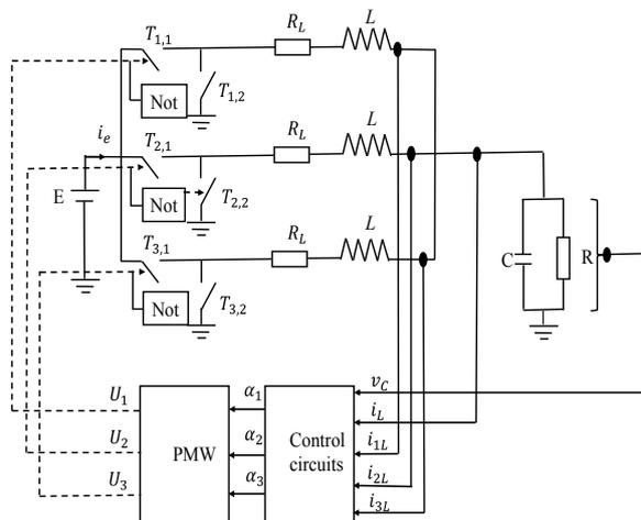
Fig.7. Multi-loop control for three parallel buck converter
