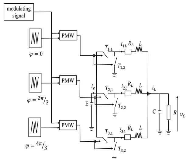
Fig.1. Three phases parallel multi-cell converter
