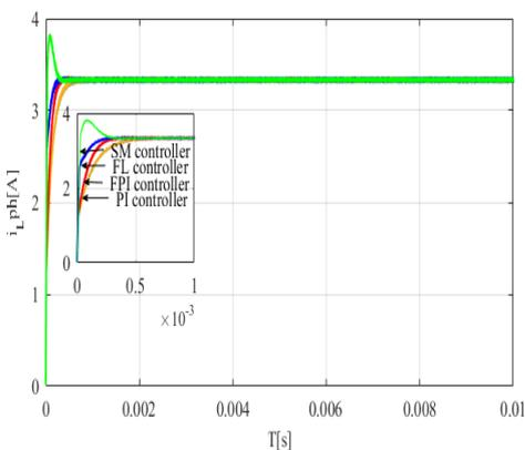
Fig.10. Phases currents of parallel multicellular Buck converter with the four controllers
