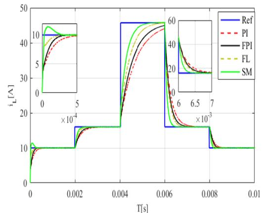
Fig.16. Dynamic responses of output current with changes in load using the controllers
