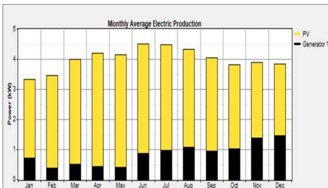
Fig.15. Statistics on the yearly electrical power production and consumption of the system
