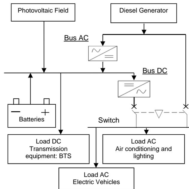
Fig.3. Hybrid system topology
