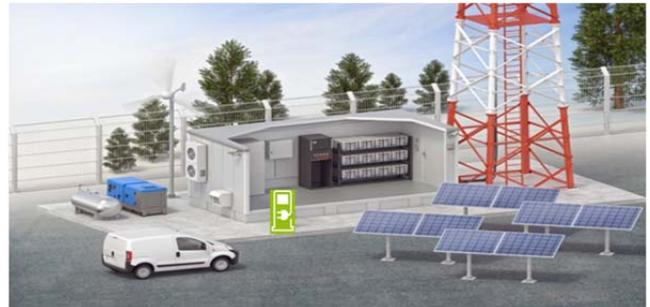
Fig.2. Configuration of system telecommunications equipment and charger for electric vehicle
