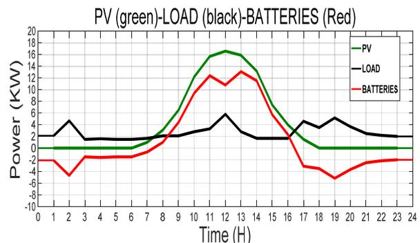
Fig.9. Graph of the Power (PV, LOAD, BATT)
