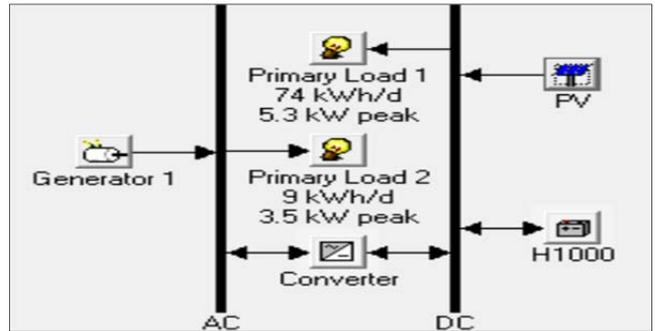
Fig.13. System architecture after entering the required data
