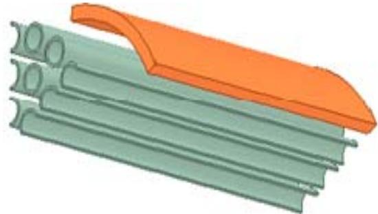
Fig. 2. Symmetrical 1/12 part of the induction system
