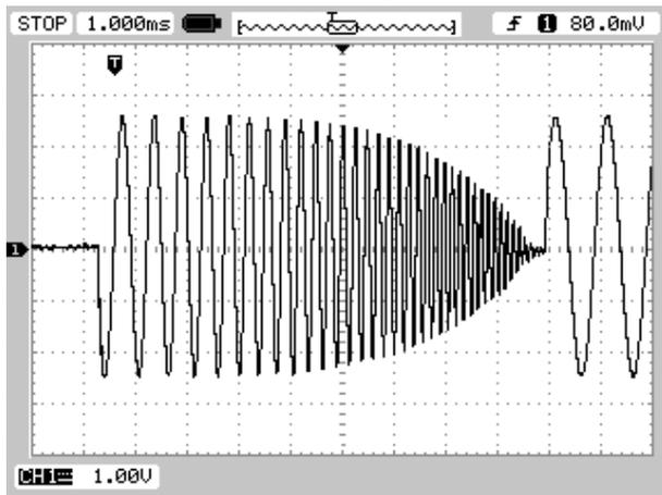
Fig.3. The oscillogram of "Pulsar" anti-aliasing LPF as response on the input sinusoidal signal with frequency sweep from 1 to 10 kHz range (exponential sweep of frequency).
