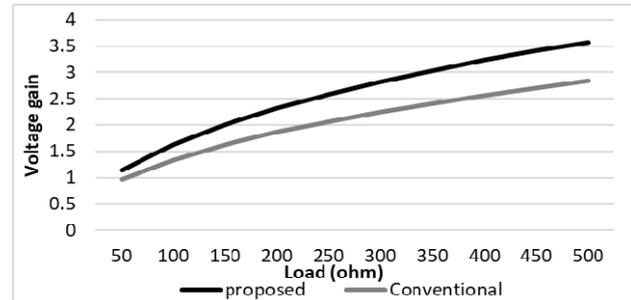
Fig. 8. Comparison of voltage gain between proposed and conventional converter for load variation ( $F_s=5\text{ kHz}$ ,  $D=0.5$ )
