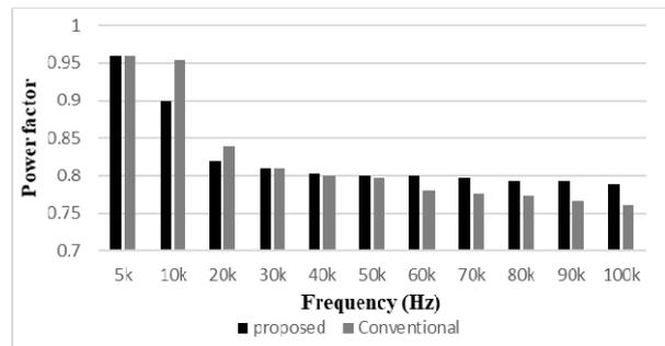
Fig. 9. Comparison of power factor between proposed & conventional converter under  $F_s$  variation ( $D=0.5$  and  $R_o=100\Omega$ )
