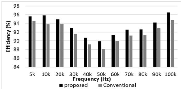
Fig. 10. Comparison of efficiency between proposed & conventional converter under  $F_s$  variation ( $D=0.5$  and  $R_o=100\Omega$ )
