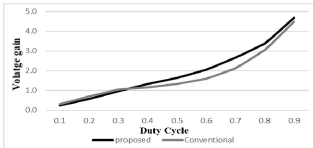
Fig. 6. Comparison of voltage gain between proposed & conventional converter for duty cycle variation ( $R_o=100\Omega$ ,  $F_s=5\text{kHz}$ )
