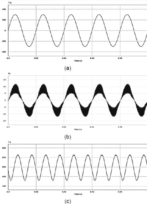
Fig 3. Waveform of (a) input voltage, (b) input current and (c) output voltage
