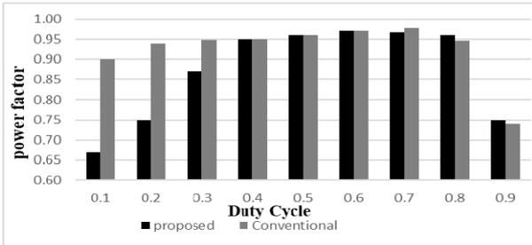
Fig. 4. Comparison of input PF between proposed and conventional converter for duty cycle variation ( $R_o=100\Omega$ ,  $F_s=5\text{ kHz}$ )
