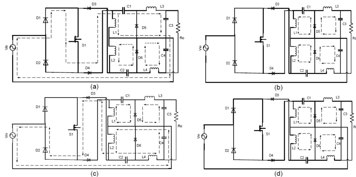
Fig. 2: Four Modes of Operation of Proposed AC-DC Zeta Converter (a) Mode 1:Proposed circuit in positive half cycle when S1 is ON.(b) Mode 2:Proposed circuit in positive half cycle when S1 is OFF. (c) Mode 3:Proposed circuit in negative half cycle when S1 is ON.(d)Mode 4:Proposed circuit in negative half cycle when S1 is OFF
