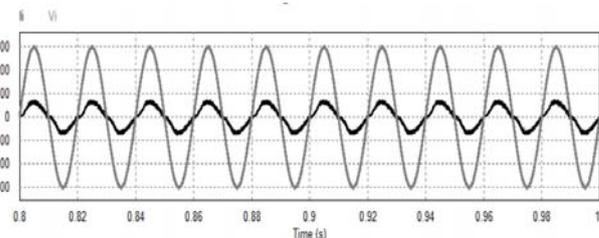
Fig. 14. Waveform of input current and input voltage for proposed converter with feedback controller
