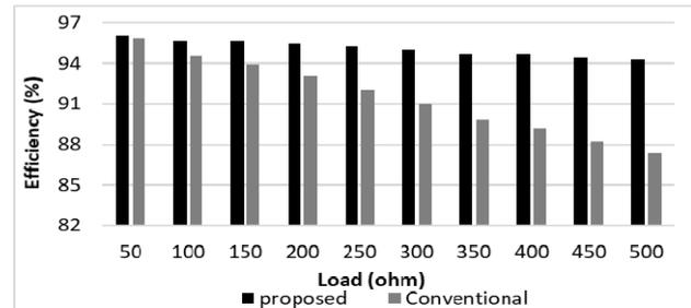
Fig. 7. Comparison of efficiency between proposed and conventional converter for load variation ( $F_s=5\text{ kHz}$ ,  $D=0.5$ )
