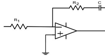
Fig. 13. PI controller for feedback operation
