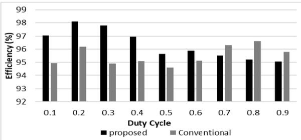
Fig. 5. Comparison of efficiency between proposed & conventional converter for duty cycle variation ( $R_o=100\Omega$ ,  $F_s=5\text{ kHz}$ )
