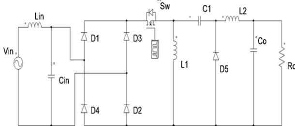
Fig.1. Proposed Single-Phase AC-DC Zeta Converter (a), Conventional Single-Phase AC-DC Zeta Converter (b)
