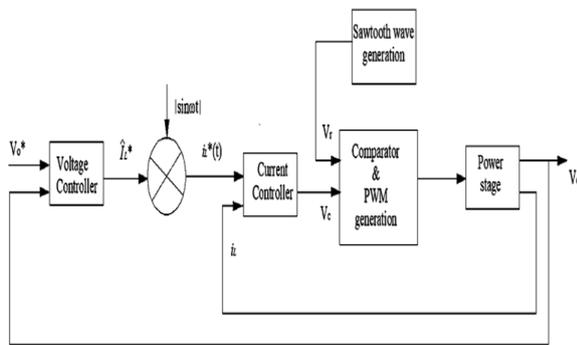
Fig. 11. Control loop for proposed feedback control system
