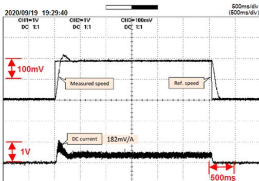
Fig. 12. Speed response 1400 rpm by PI control using GA
