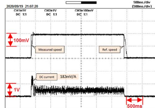
Fig. 14. Speed response 1400 rpm by PI control using ACO
