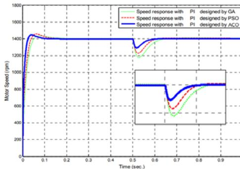
Fig.9. The speed response simulation by PI control using GA, PSO and ACO controller
