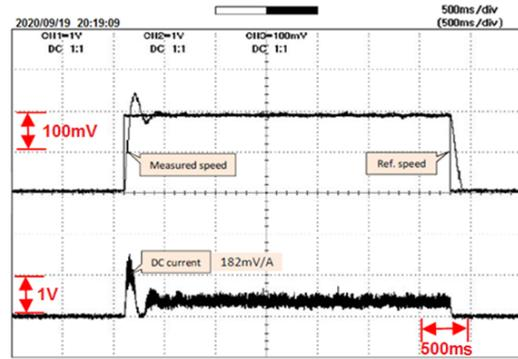
Fig. 13. Speed response 1400 rpm by PI control using PSO
