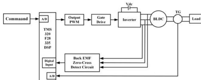
Fig. 2. DSP-based BLDC motor speed control system
