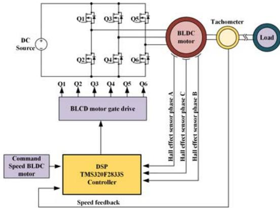
Fig. 3. The proposed BLDC motor speed control system.
