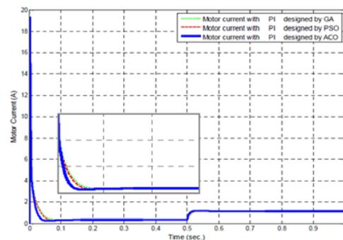
Fig.10. The currents response simulation by PI control system using GA, POS, and ACO controller
