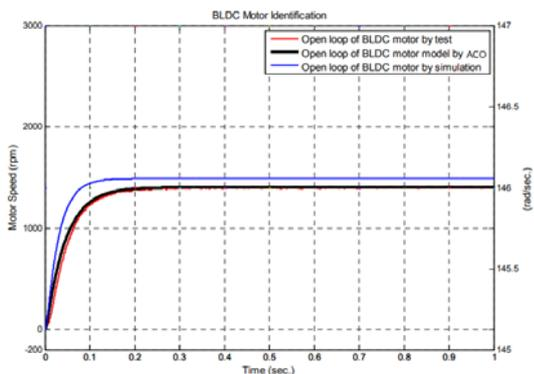
Fig. 7. The open-loop response of a BLDC motor at 1400 rpm.
