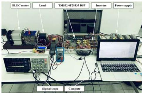
Fig. 11. BLDC motor experimental setup
