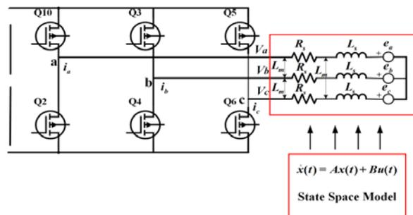
Fig. 2. The designing state space model of BLDC motor connected to an inverter.
