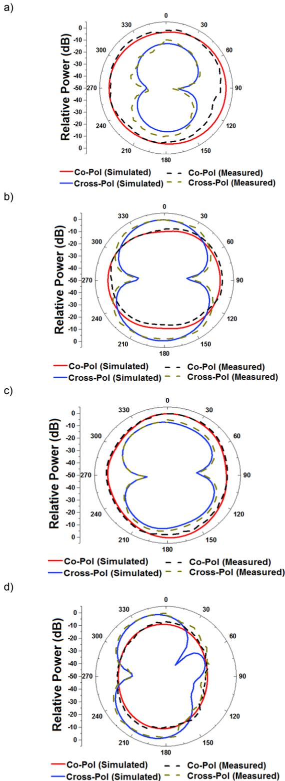
Fig.10. Normalized radiation patterns(a)at 3.5 GHz in x-z plane (b) at 3.5 GHz y-z plane (c) at 5.5 GHz in x-z plane and (d) at 5.5 GHz in y-z plane
