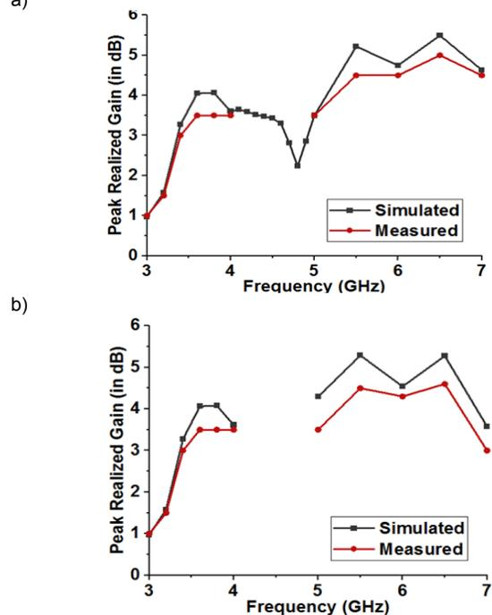
Fig.9. Peak realized Gain when PIN diode (a) ON condition and (b) OFF condition
