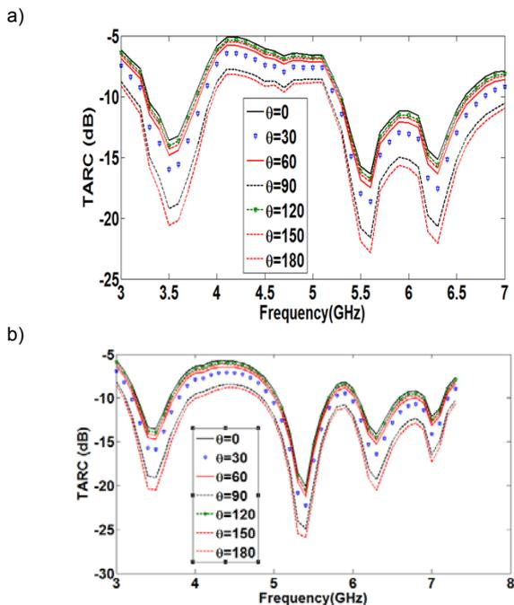
Fig.13. TARC when PIN diode (a) ON condition and (b) OFF Condition
