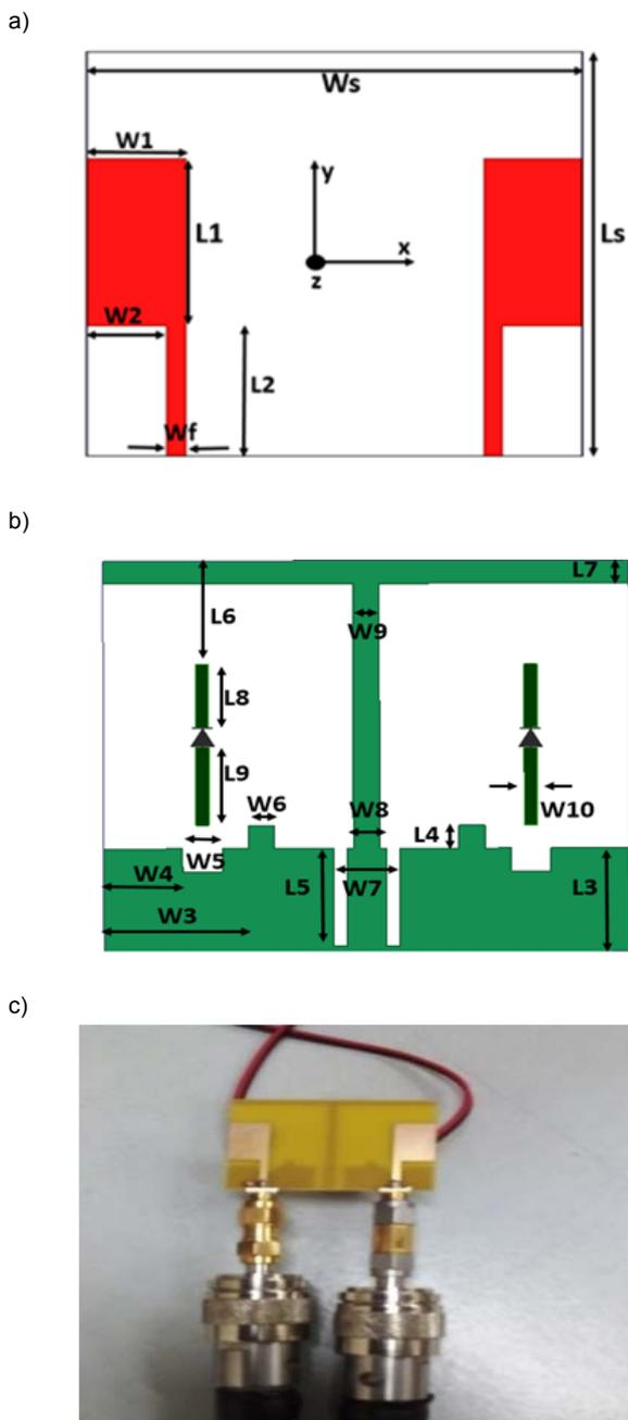
Fig.1. Designing of proposed two port antenna (a) in front view (b) bottom view with parasitic patch and (c) prototype
