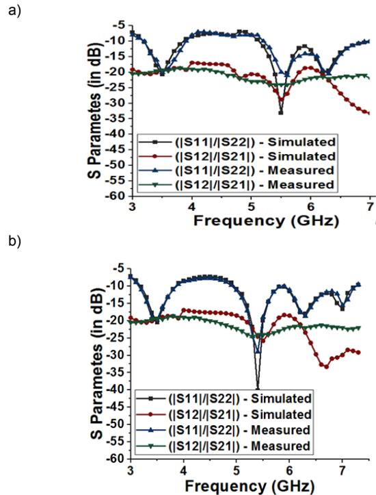
Fig 8 S-parameter and isolation curve of the proposed two-port antenna when PIN diode (a) ON condition and (b) OFF condition
