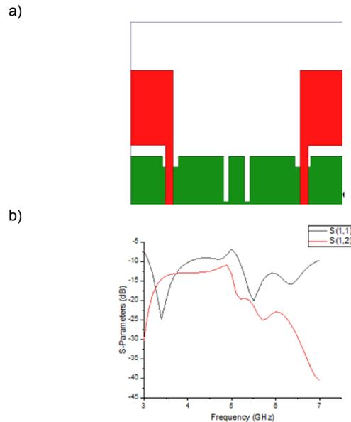
Fig4. (a) Step-3 designing of two port antenna and (b) S parameters and isolation curve
