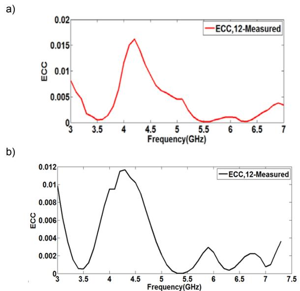
Fig.11. ECC when PIN diode (a) ON state and (b) OFF state
