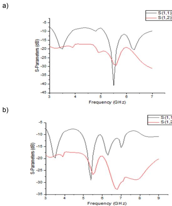
Fig 6 Simulated S-parameter and isolation curve of the proposed antenna when PIN diode (a) ON Condition and (b) OFF Condition
