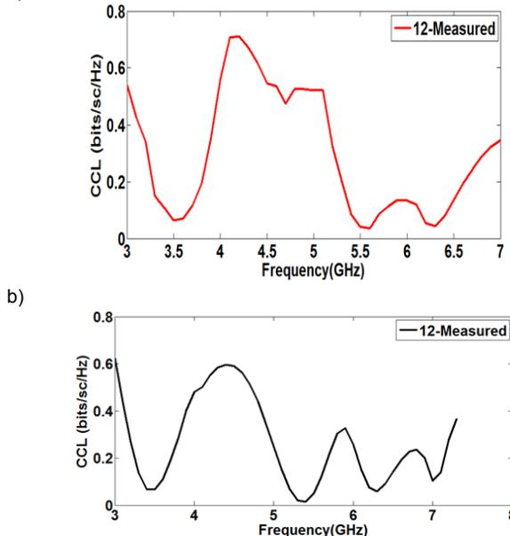
Fig.14. CCL when PIN diode (a) ON condition and (b) OFF condition
