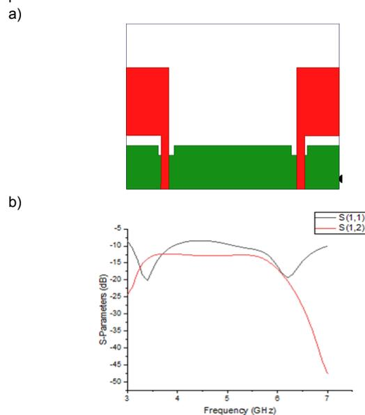
Fig3. (a) Step-2 designing of two port antenna and (b) S parameters and isolation curve
