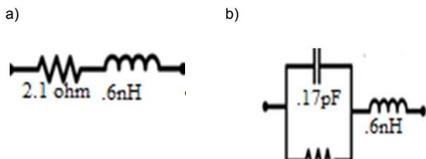
Fig.7. Equivalent circuit of PIN diode when (a) ON state and (b) OFF state
