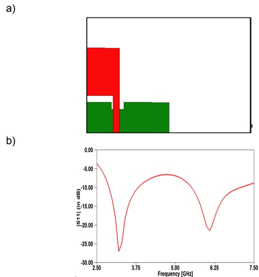
Fig2. (a) Step-1 designing of single element antenna and (b) S parameters
