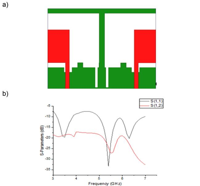
Fig.5. (a) Step-4 designing of a two-port antenna with T stub and (b) S-parameters and isolation curve
