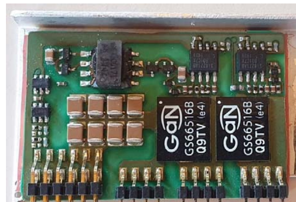
Fig. 2. Tested prototype – isolated metal substrate board with GaN (GS66516B) half-bridge and insulated gate drivers
