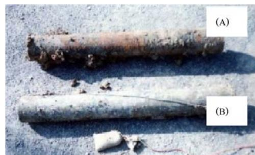
Fig. 17. Results of the structural comparison of the non-corrosion-protected pipes (A) with the impressed current corrosion protection metal pipes (B).
