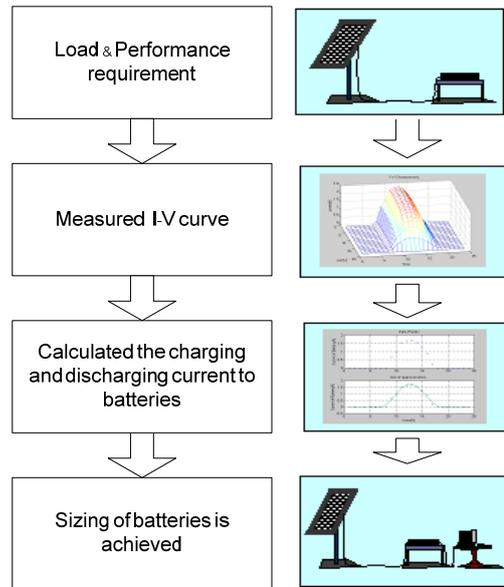
Fig. 3. Order of each part of the procedure for analyzing the solar power systems according to the proposed method.
