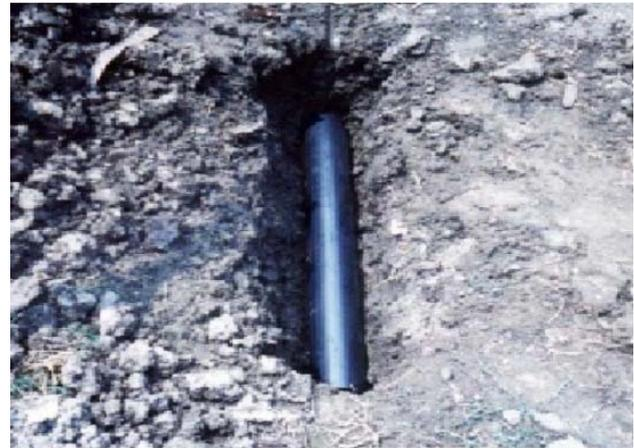
Fig. 13. The metal pipe used for the impressed current corrosion protection test.
