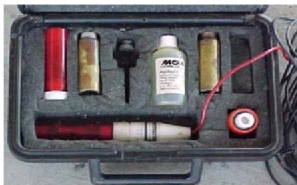
Fig. 16. The Cu/CuSo 4 probe for measuring the anti-corrosion performance of the metal pipes.
