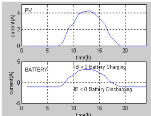
Fig. 7. The results of showing the current values at each time of the solar power system.
