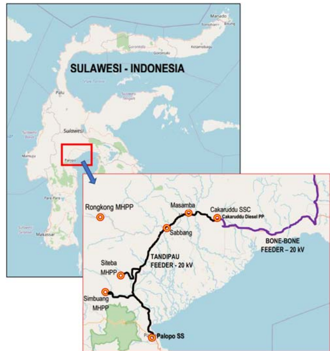
Fig. 3. Location of Rongkong MHPP and Tandipau Feeder
