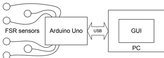
Fig. 7. Block diagram of presented posture measurement solution.
