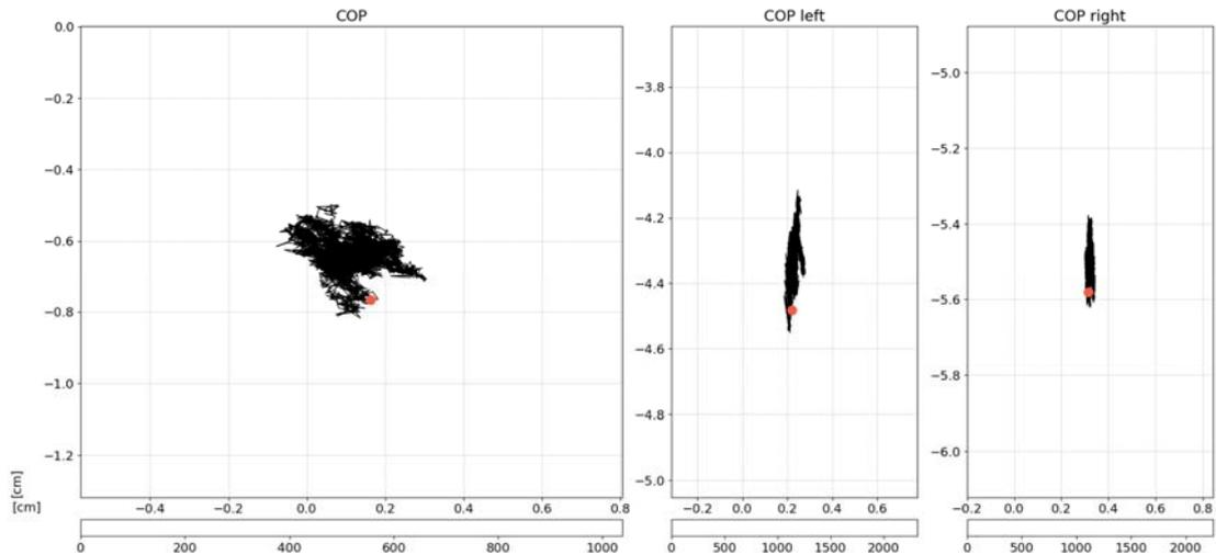
Fig. 12. Stabilogram of the test for a person with open eyes.
