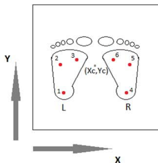
Fig. 1. The center of pressure detection.
