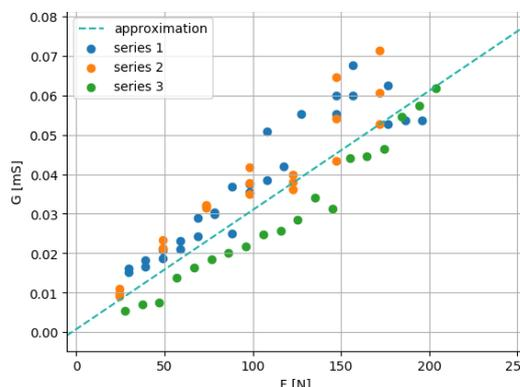
Fig. 4. Fitting curve of Conductance vs force for 20kg FSR sensor.
