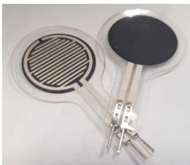
Fig. 2 Force-Sensing Resistor.
