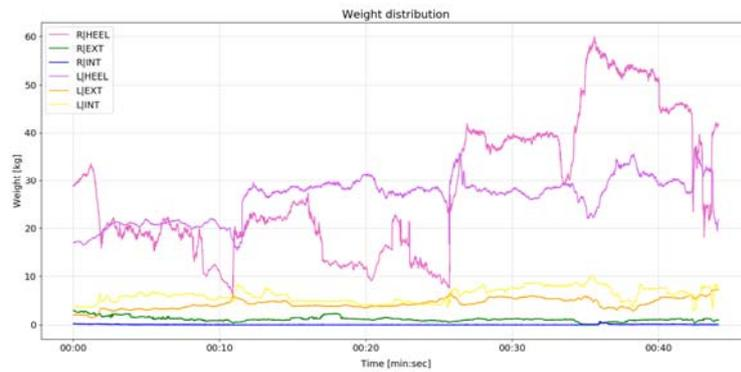
Fig. 11. Visualization of the load on the sensors over time (test of a person holding a weight of 8 kg).
