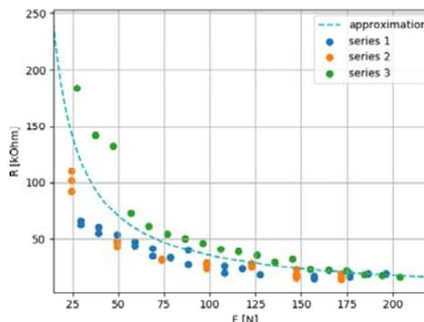
Fig. 3. Fitting curve of resistance vs force for 20kg FSR sensor.
