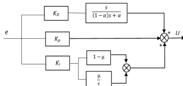
Fig.1. Block diagram of the fractional order regulator for which the integral component obtained on the basis of the Laplace image of the fractional order derivative using the Caputo-Fabrizio operator.
