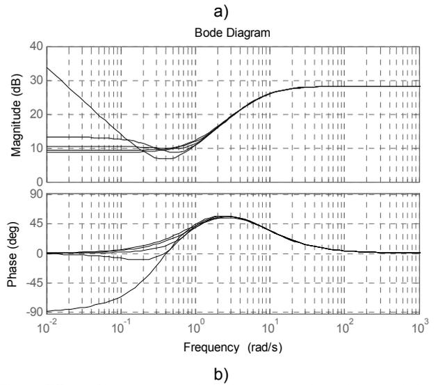
Fig. 5. Effect of parameter  $\mu$  changing on transient characteristic of system and frequency characteristics in case of the fractional controller
