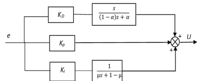
Fig.2. Block diagram of the fractional order PID-controller obtained using an integrated operator with a non-singular core [20].
