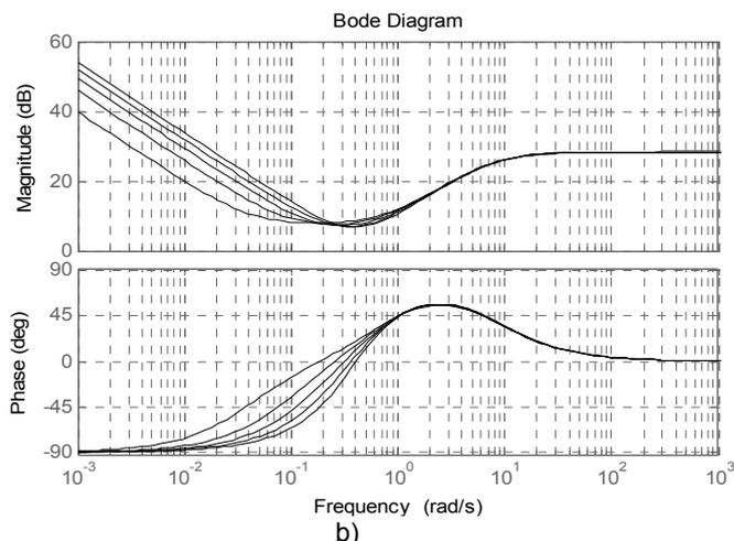
Fig. 3. Effect of parameter  $\mu$  changing on transient characteristic of system and frequency characteristics in case of the fractional controller
