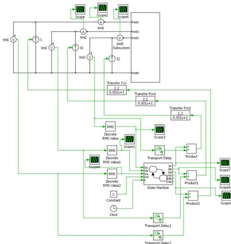
Fig.3. PLECS compensator model with current controlled sources
