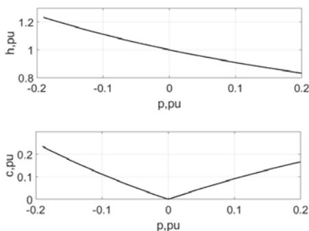
Fig.2. Voltage gain  $h$  and compensator current  $c$  as functions of control parameter  $p$
