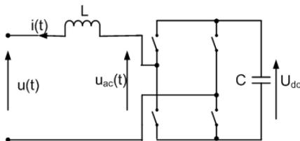
Fig. 9. General structure of the inverter
