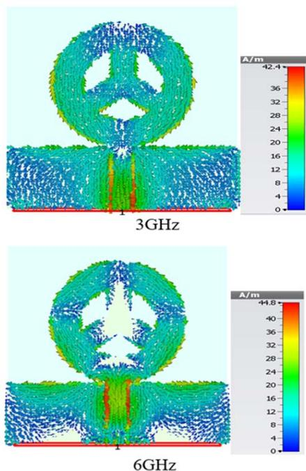
Fig.5. The surface current flow at different frequencies
