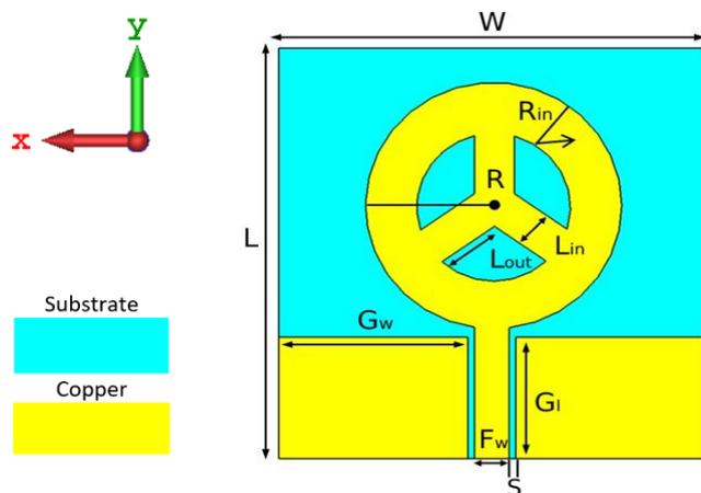
Fig. 1. The geometry of the proposed MPM antenna
