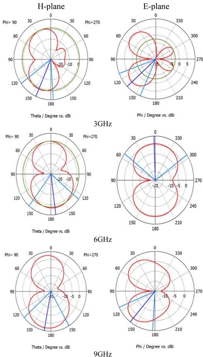
Fig. 4. The simulated radiation pattern for H and E-plane at 3GHz, 6GHz and 9GHz
