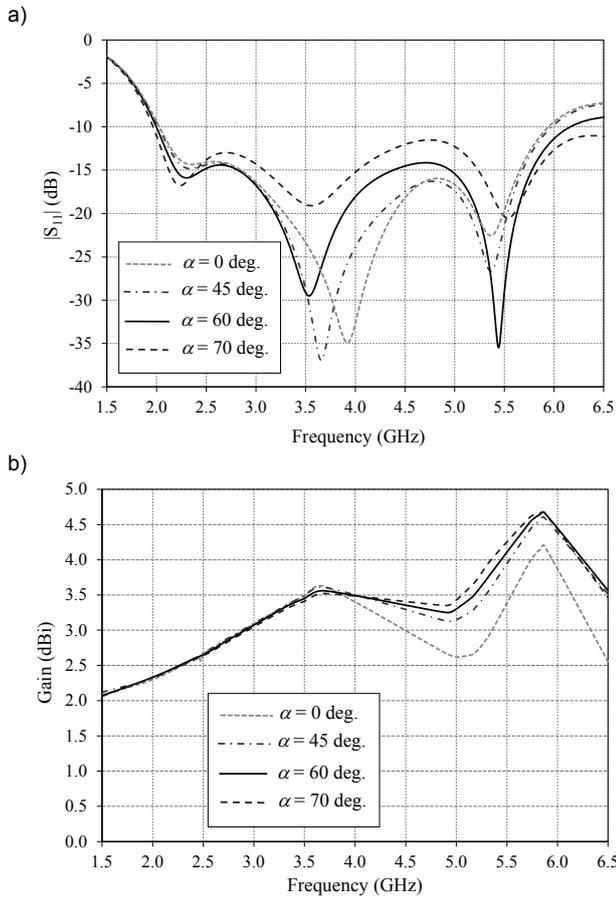
Fig.4. The effect of  $\alpha$  to : a)  $|S_{11}|$  and b) gain
