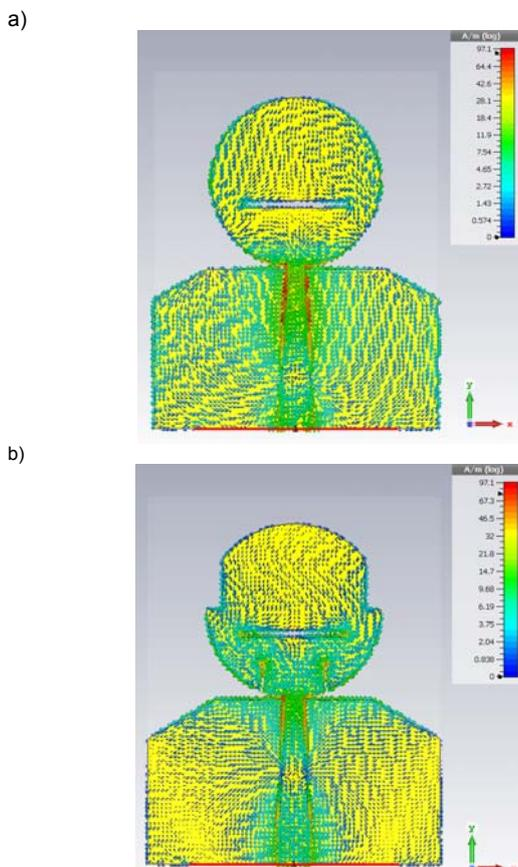
Fig.5. Surface current densities of the proposed antenna: a) without ISNS, b) with ISNS
