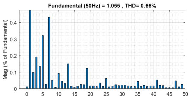
Fig. 15. Amplitude-frequency spectrum of wind turbines output voltage, determined by simulation
