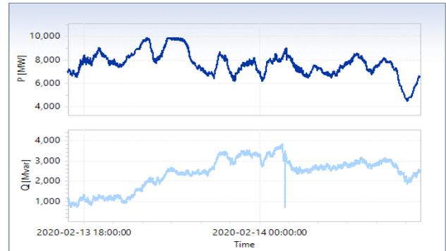
Fig. 12. Active and reactive power changes in 35 kV network on 9<sup>th</sup> interval
