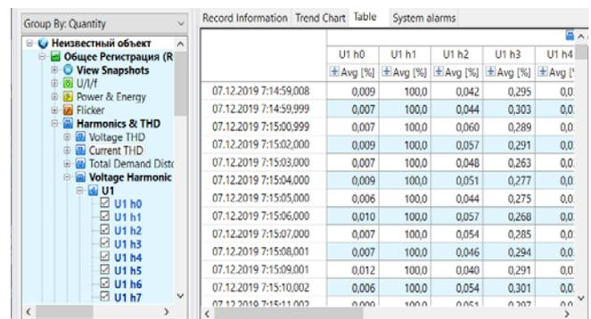
Fig. 2. Table amplitudes of higher harmonics of phase voltage
