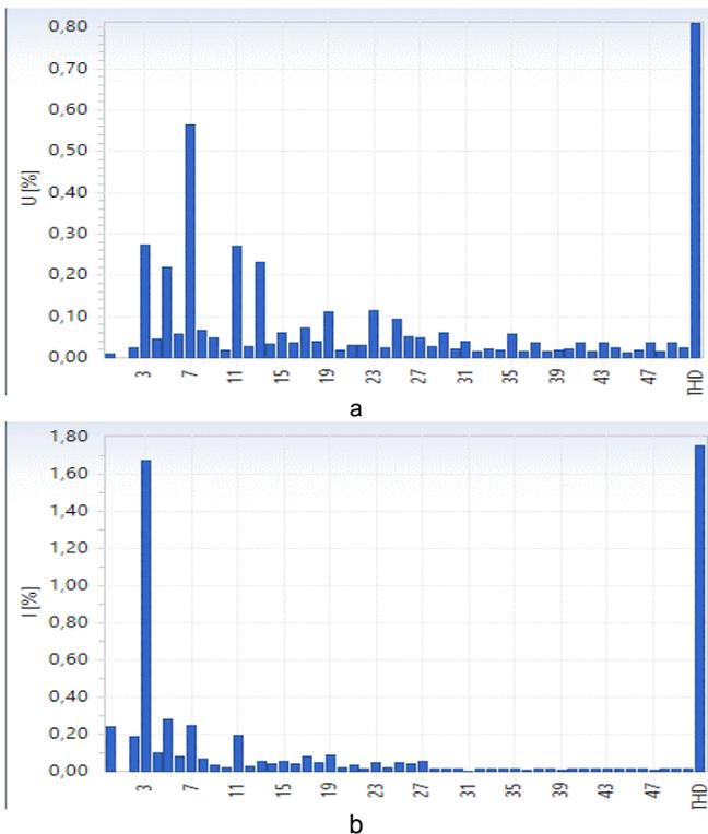
Fig. 11. Example of 35 kV individual harmonic voltage (a) and current (b) values
