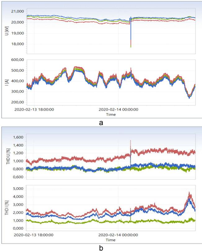
Fig. 10. Graphs of 35 kV voltages and currents on 3 interval (a) and the corresponding graphs of voltages and currents THD (b)
