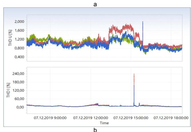
Fig. 6. Graphs of 150 kV voltages and currents on 3 interval (a) and the corresponding graphs of voltages and currents THD (b)
