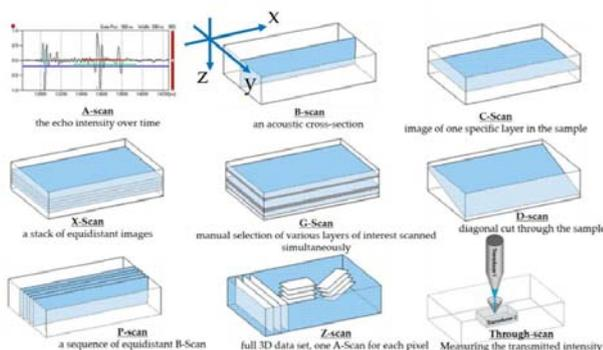
Fig.9: Scan modes of SAM (image courtesy of PVA TePla Analytical Systems) [29].
