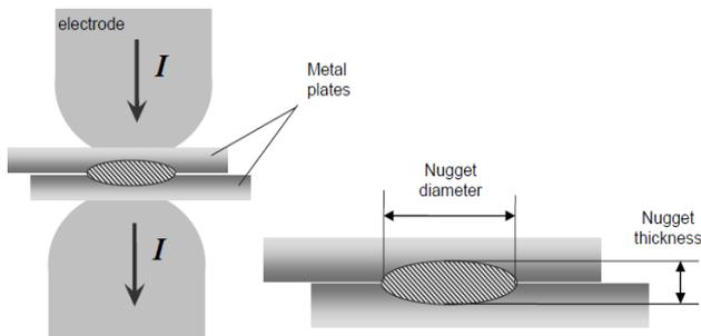
Fig. 2: Resistance welding process and weld structure [16]
