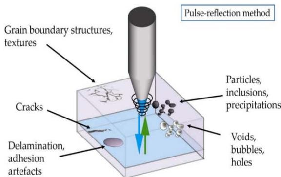
Fig.8: Defect detection and sample interaction (image courtesy of PVA TePla Analytical Systems) [29].
