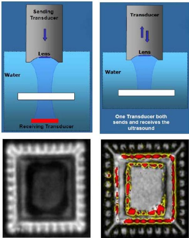
Fig.5: Differential between Reflection Mode (C-Scan) - right and Transmission Mode (Thru-Scan) - left (a) Schematic diagram, (b) image
