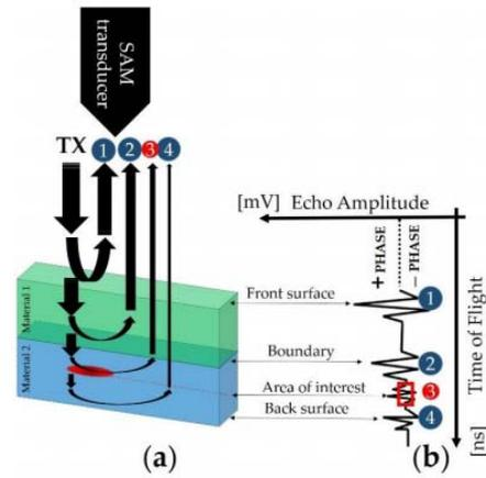
Fig.7: A-scan through the thickness of the sample under testing (target object) [27].
