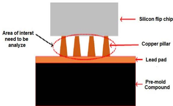
Fig.6: Schematic diagram of flip chip package internal construction.
