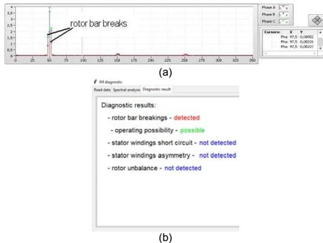
Fig. 7 Diagnostic for IM with the broken rotor bar
