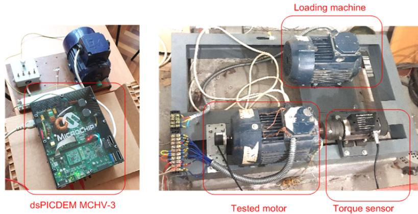
Fig. 6 Laboratory equipment appearance
