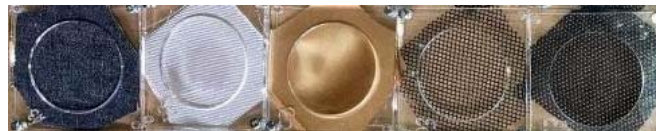
Fig. 2. Samples of knitted fabrics: denim, glass fiber, silk, two different non-woven fabric
