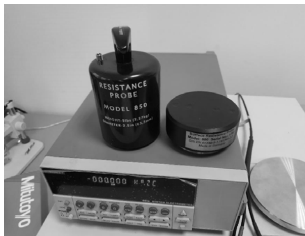
Fig.6. Laboratory stand for resistance measurement
