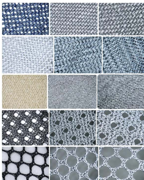
Fig.5. Textiles without aluminum coating, with one coating layer, and with five coating layers
