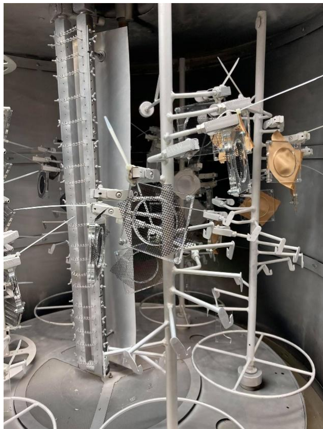
Fig. 4. Assembly of samples in the metallizer chamber
