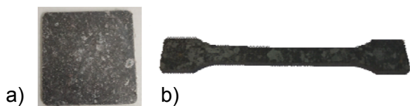
Fig. 1. Samples used in the carried out tests in shape of square plates (a) and paddles (b)
