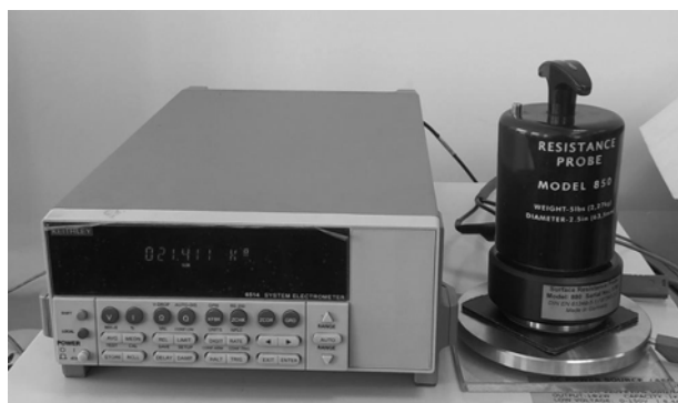
Fig. 2. Test bench used for measurement of the volume resistance
