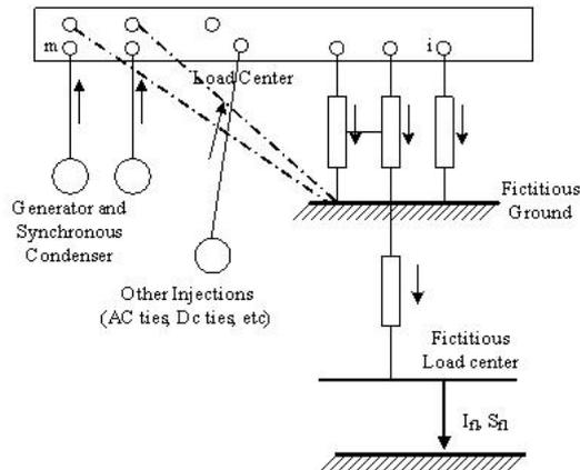
Fig. 4. Zero Power Balance Network
