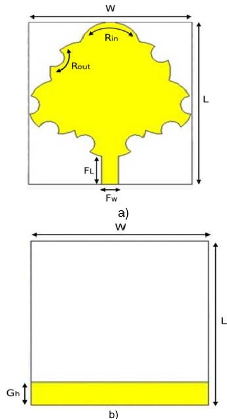
Fig. 1. Antenna parameters in both (a) Front view and (b) Back view.
