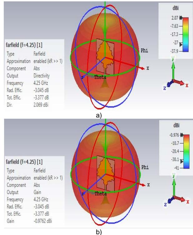
Fig. 4. Simulated results of the suggested antenna (a) Directivity and (b) Gain.
