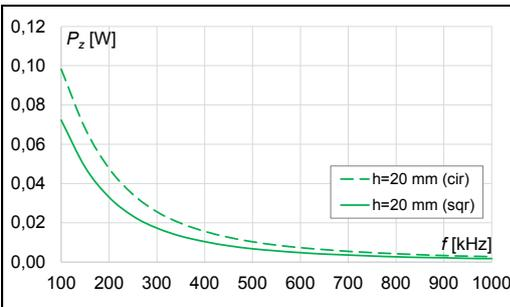
Fig. 15. Results of transmitter power ( $P_z$ ) dependent of kind of coils, number of turns ( $n=70$ ) at distance ( $h=20$  mm)
