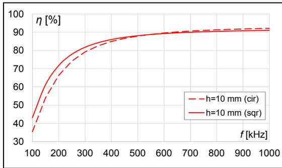
Fig.8. Results of transfer efficiency ( $\eta$ ) dependent of kind of coils, number of turns ( $n=30$ ) at distance ( $h=10$  mm)
