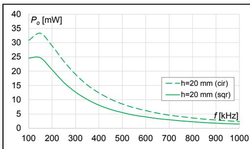
Fig. 16. Results of receiver power ( $P_o$ ) dependent of kind of coils, number of turns ( $n=70$ ) at distance ( $h=20$  mm)
