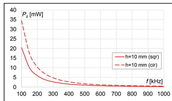
Fig.12. Results of transmitter power ( $P_z$ ) dependent of kind of coils, number of turns ( $n=70$ ) at distance ( $h=10$  mm)
