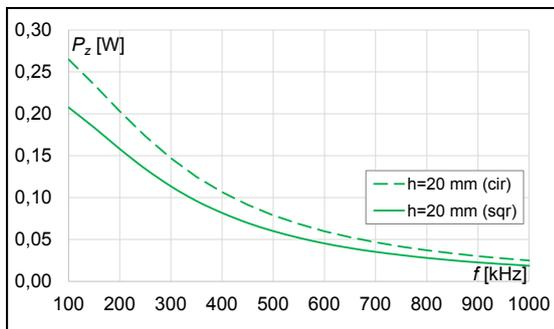
Fig.9. Results of transmitter power ( $P_z$ ) dependent of kind of coils, number of turns ( $n=30$ ) at distance ( $h=20$  mm)
