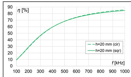
Fig.11. Results of transfer efficiency ( $\eta$ ) dependent of kind of coils, number of turns ( $n=30$ ) at distance ( $h=20$  mm)
