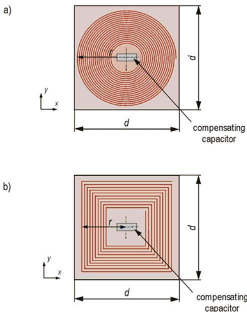
Fig.3. The types of coils considered in the models of WPT system: a) circular coil, b) square coil
