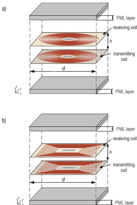
Fig.5. A numerical three-dimensional model of WPT cell for: a) circular coils, b) square coils
