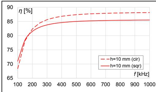
Fig. 14. Results of transfer efficiency ( $\eta$ ) dependent of kind of coils, number of turns ( $n=70$ ) at distance ( $h=10$  mm)
