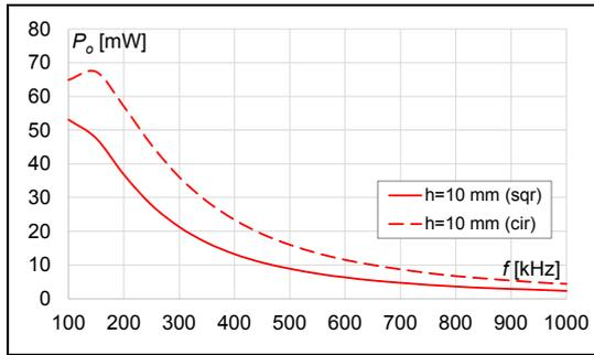
Fig.7. Results of receiver power ( $P_o$ ) dependent of kind of coils, number of turns ( $n=30$ ) at distance ( $h=10$  mm)
