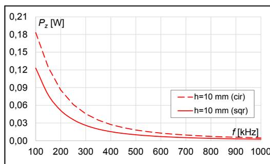
Fig.6. Results of transmitter power ( $P_z$ ) dependent of kind of coils, number of turns ( $n=30$ ) at distance ( $h=10$  mm)
