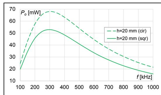
Fig.10. Results of receiver power ( $P_o$ ) dependent of kind of coils, number of turns ( $n=30$ ) at distance ( $h=20$  mm)
