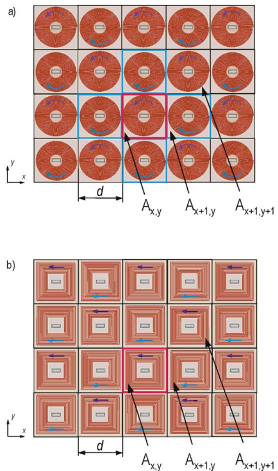
Fig.4. A two-dimensional set transmitting/receiving surface of the checkerboard type WPT system for: a) circular coils ( $A_{x,y}$  – the WPT cell), b) square coils
