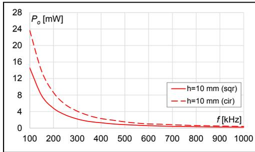
Fig. 13. Results of receiver power ( $P_o$ ) dependent of kind of coils, number of turns ( $n=70$ ) at distance ( $h=10$  mm)
