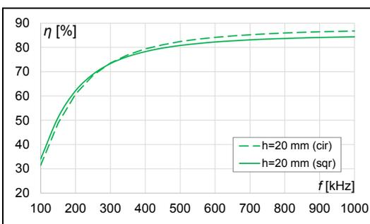
Fig. 17. Results of transfer efficiency ( $\eta$ ) dependent of kind of coils, number of turns ( $n=70$ ) at distance ( $h=20$  mm)
