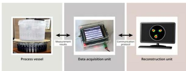
Fig.1. Measurement model for ultrasound tomography
