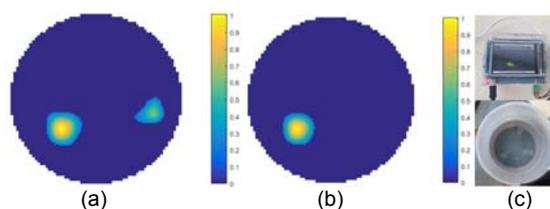
Fig.3. Examples of reconstruction using ultrasound tomography for 20 measuring points with 48 kHz transducers: (a) image reconstruction for 2 objects, (b) image reconstruction for 1 object, (c) tomographic system
