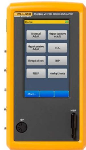
Fig.2. FLUKE model ProSim 4 ECG simulator [30].
