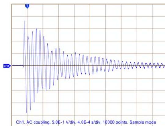
Fig. 4. Waveform of the signal generated by the piezoelectric plate
