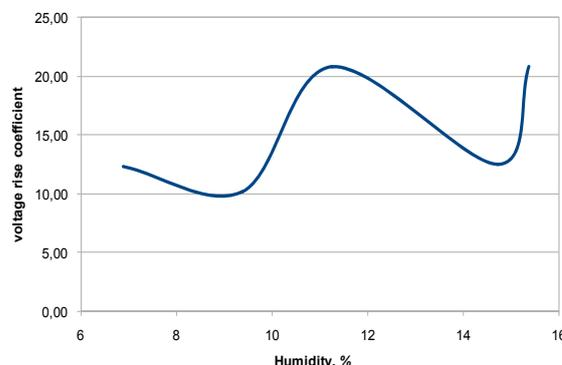
Fig. 5. The value of the voltage rise coefficient on the piezoelectric transducer for Mung beans
