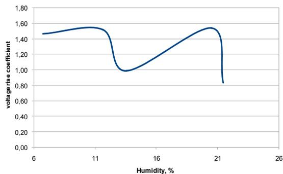
Fig. 6. The value of the voltage rise coefficient on piezoelectric transducer for coriander seeds
