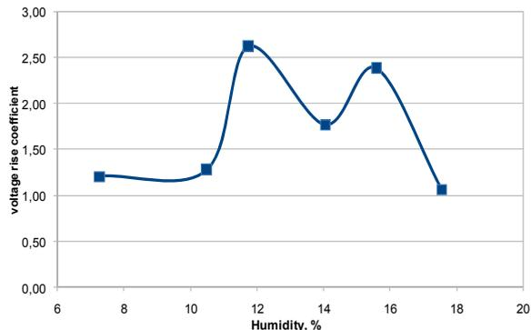
Fig. 7. The value of the voltage rise coefficient on the piezoelectric transducer for hemp seeds
