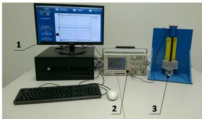
Fig. 1. Test stand: 1 – computer processing the signal, 2 – oscilloscope; 3 – measuring system
