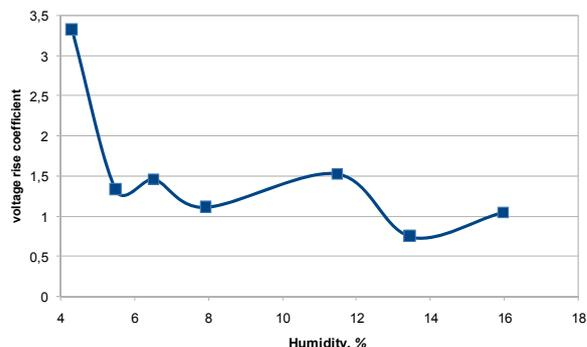
Fig. 9. The value of the voltage rise coefficient on the piezoelectric transducer for for mustard
