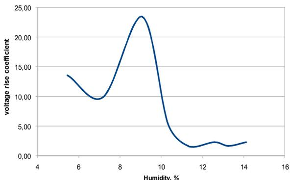
Fig. 8. The value of the voltage rise coefficient on the piezoelectric transducer for millet seeds
