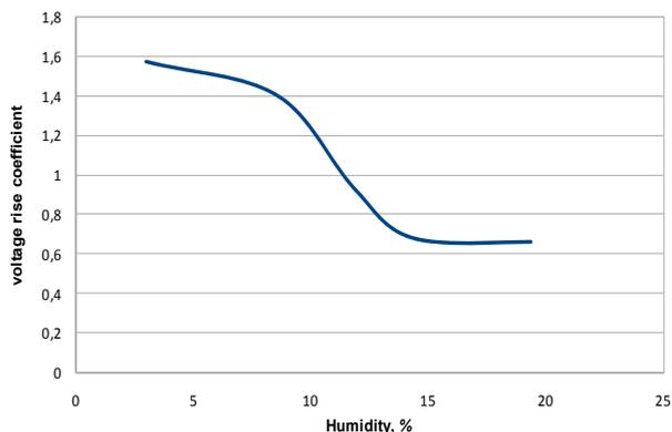
Fig. 10. The value of the voltage rise coefficient on the piezoelectric transducer for rape
