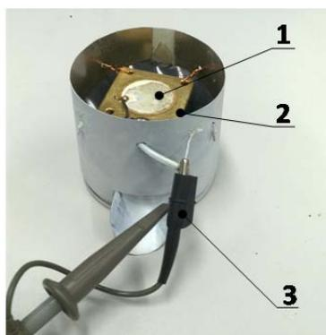
Fig. 2. The measuring system: 1 – piezoelectric plate, 2 – plate suspension, 3 – cable leads to the oscilloscope
