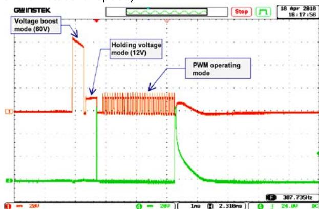
Fig.4. Time courses of voltages on (transistor drain) controlling the operation of the injector in the Audi A3 vehicle
