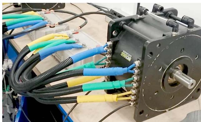
Fig.7. View of the test stand: with a BLDC motor (HPM-20 kW) powered from the converter
