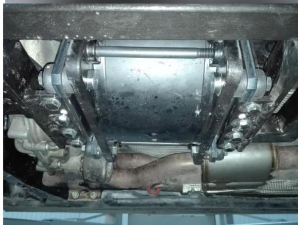
Fig.8. Design (3D model) of the drive mounting in the VW Touareg and below the final result of the work in a mechanical workshop
