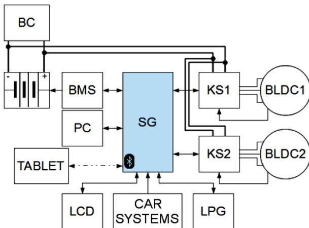
Fig.3. Block diagram of the control structure of a hybrid system
