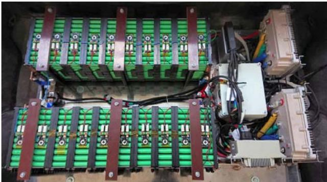
Fig.9. The battery pack installed in the vehicle with engine controllers
