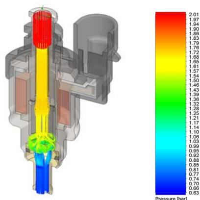
Fig.1. Gas flow trajectory through the injector (longitudinal section view)
