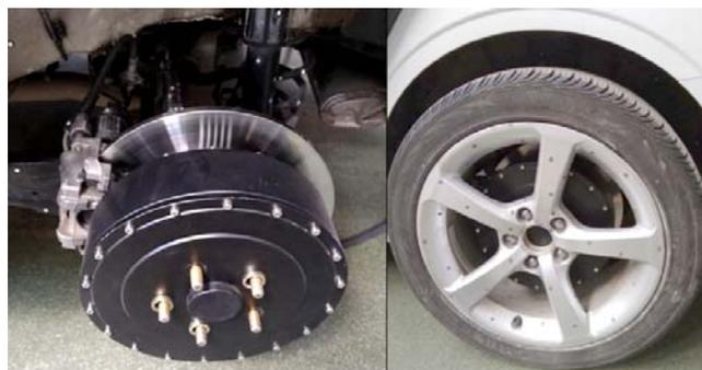
Fig.6. The way of mounting the BLDC drive in the rear wheel hub - Audi A3
