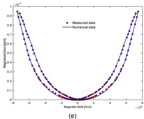
Fig.5. Magnetostriction curves versus magnetic field at different compressive stress values. (a) 0MPa. (b)-6MPa. (c)-12MPa. (d)-18MPa. (e)-24MPa
