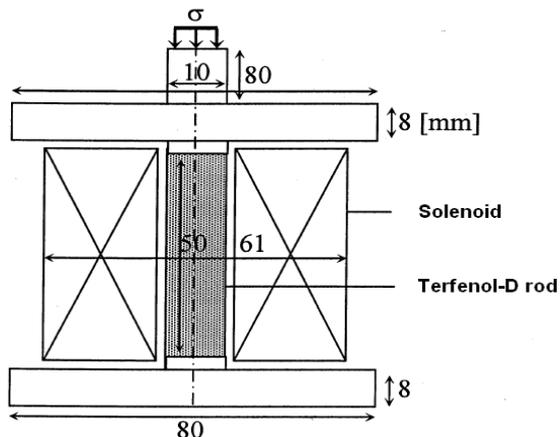
Fig.4. Schematic diagram of the magnetostrictive device
