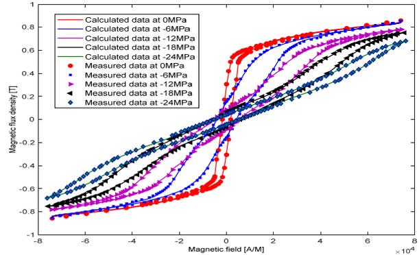
Fig.2. Hysteresis curves for different compressive stress values.
