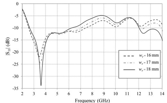
Fig.3.  $|S_{11}|$  of proposed antenna for various  $w_r$
