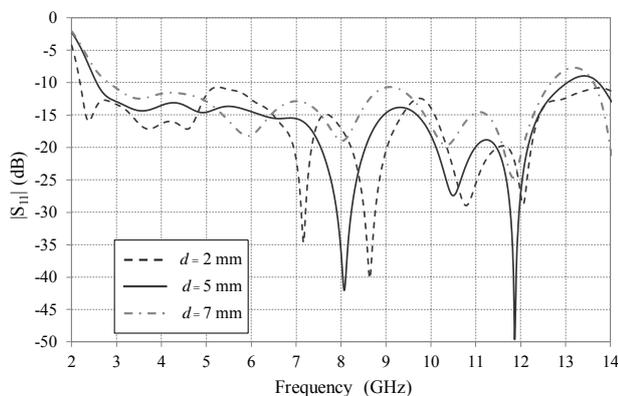
Fig.5.  $|S_{11}|$  of proposed antenna for various  $d$
