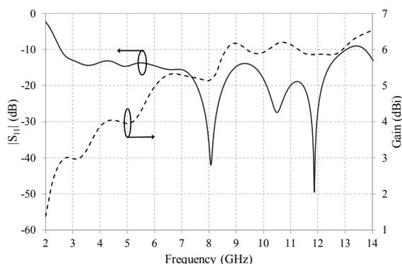
Fig.7.  $|S_{11}|$  and gain of proposed antenna
