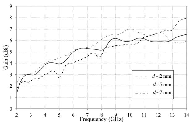
Fig.6. Gain of proposed antenna for various  $d$
