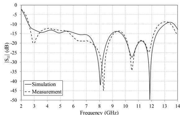
Fig.8. Simulated and measured  $|S_{11}|$
