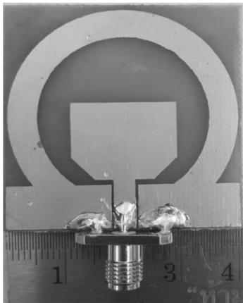
Fig.1. Geometry of the proposed antenna: a) its model and b) photo of its prototype
