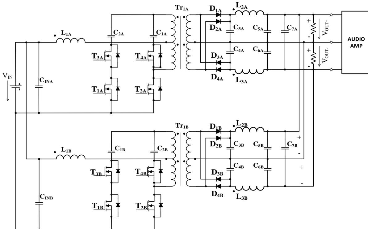
Fig.1. Principal schematics of the proposed current fed interleaved push-pull converter with active clamp for automotive audio amplifier system
