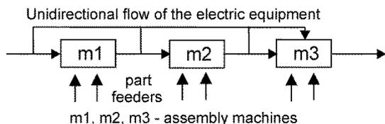
Figure 1. Example of diagram of assembly line without buffers
