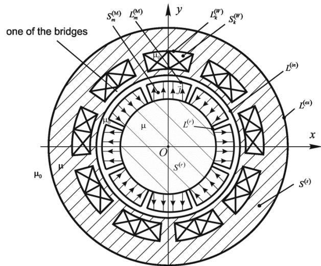
Fig. 1. The electric motor cross section with a smooth stator
