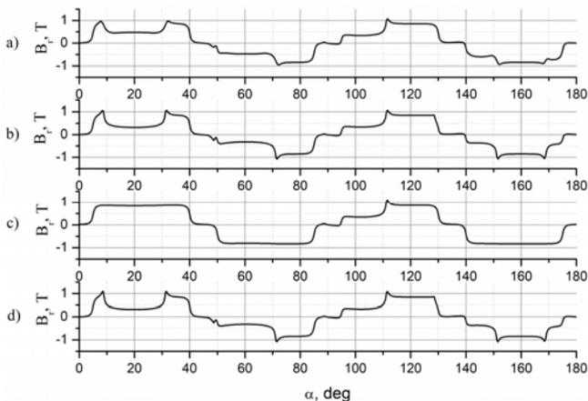
Fig. 3. Graph of magnetic induction r-components distribution in the working gap between the rotor and the stator
