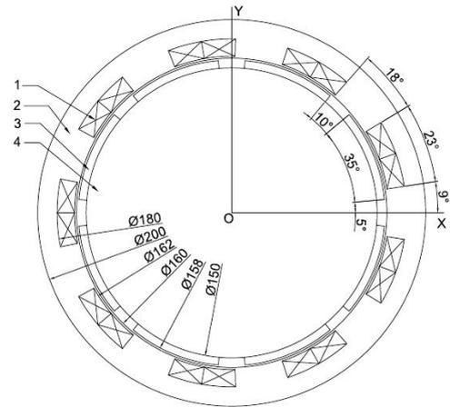
Fig. 2. The geometric parameters of the electric motor
