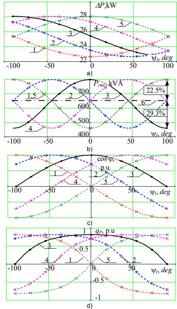
Fig. 2. Change of the indicators depending on the change of the current initial phase: a) line power loss; b) the load power RMS norm is ratio to apparent power; c) the generalized coefficient of power symmetry; d) active power degree. (1 – voltage phase shift  $-90^\circ$ , 2 – voltage phase shift  $-45^\circ$ , 3 – voltage phase shift  $0^\circ$ , 4 – voltage phase shift  $45^\circ$ , 5 – voltage phase shift  $90^\circ$ ).
