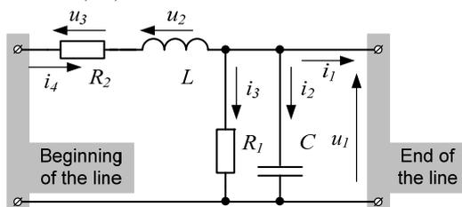
Fig. 1. Transmission line equivalent circuit
