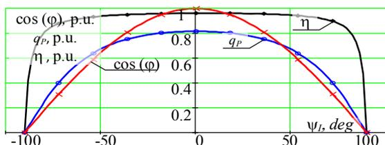
Fig. 3 The dependence of the power factor, active power amount and the efficiency of the line on the current phase shift
