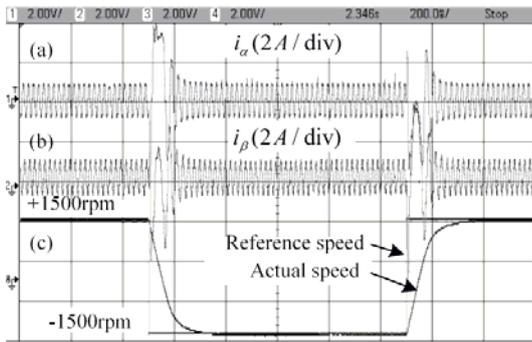
Fig. 13. Forward and reverse direction at  $\pm 1500$  rpm (a) stator current  $i_\alpha$  (b) stator current  $i_\beta$  (c) reference and actual speed.
