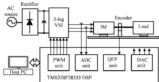
Fig. 9. Overall system for implementation.
