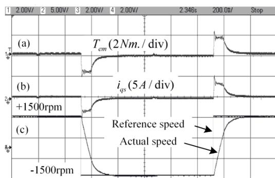
Fig. 11. Forward and reverse direction at  $\pm 1500$  rpm (a) electromagnetic torque  $T_{em}$  (b) torque-producing current  $i_{qs}$  (c) reference and actual speed.
