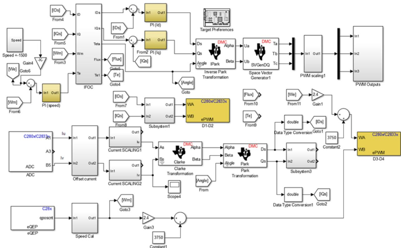
Fig. 10. MATLAB/Simulink for indirect rotor flux orientation system.
