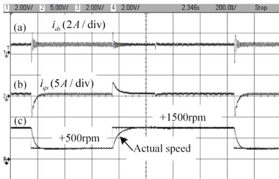
Fig. 15. Reducing and increasing speed at +500 to +1500rpm (a) flux-producing current  $i_{ds}$  (b) torque-producing current  $i_{qs}$  (c) reference and actual speed.
