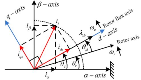
Fig. 3. Position of rotor flux vector for indirect FOC control.
