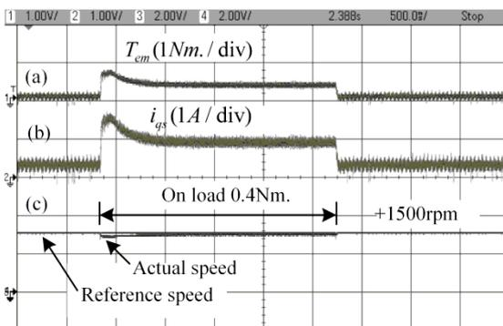
Fig. 16. A disturbed load torque condition (a) Electromagnetic torque (b) torque-producing current  $i_{qs}$  (c) reference and actual speed.
