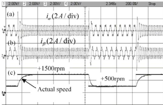
Fig. 14. Decrease and increase speed of +500 to +1500rpm (a) stator current  $i_\alpha$  (b) stator current  $i_\beta$  (c) reference and actual speed.
