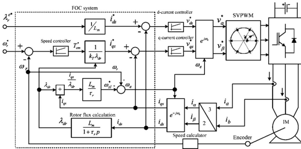
Fig. 4. Schematic block diagram of indirect rotor flux orientation system (IFOC).
