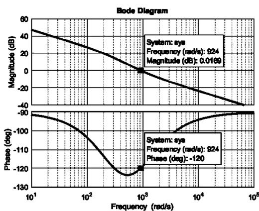
Fig. 7. Bode plot of IFOC system for current control loops.
