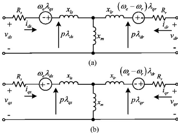
Fig. 2. Equivalent circuit in rotating reference frame.
