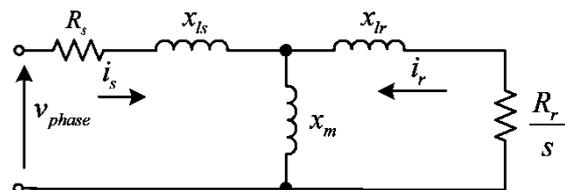
Fig. 5. Equivalent circuit of 3-phase motor per phase.
