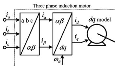
Fig. 1. Three-phase induction motor in d-q frame.
