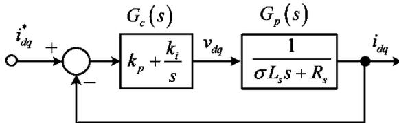
Fig. 6. Block diagram of d-q current loop controller.
