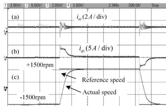
Fig. 12. Forward and reverse direction at  $\pm 1500$  rpm (a) flux-producing current  $i_{ds}$  (b) torque-producing current  $i_{qs}$  (c) reference and actual speed.
