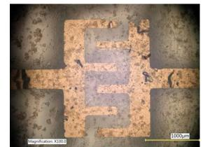
Fig. 5. Nickel capacitor electrode with cells after made experiment (magnification ×100)
