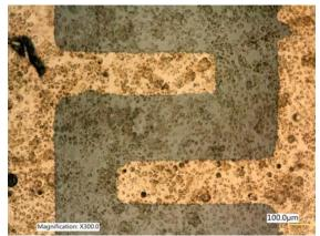
Fig. 6. Nickel capacitor electrode with cells after made experiment (magnification ×300)
