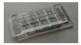
Fig. 2. Test matrix for measuring bioimpedance with eight-chamber ibidi GmbH plate with polymer bottom, compatible with ECIS measuring system.
