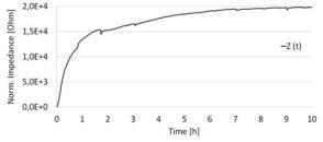
Fig. 4. Impedance response measured by a nickel sensor array at 2kHz for 18 hours.
