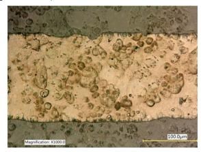
Fig. 7. Nickel capacitor electrode with cells after made experiment (magnification ×1000)
