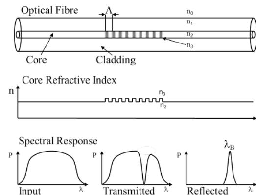
Fig.1. The principle of operation of FBG
