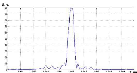
Fig. 4. The reflection spectrum of the apodized Bragg grating
