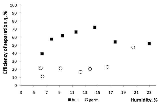
Fig. 4. Efficiency of separation as a function of humidity
