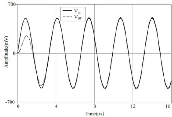
Fig.8. The transient response of bandpass
