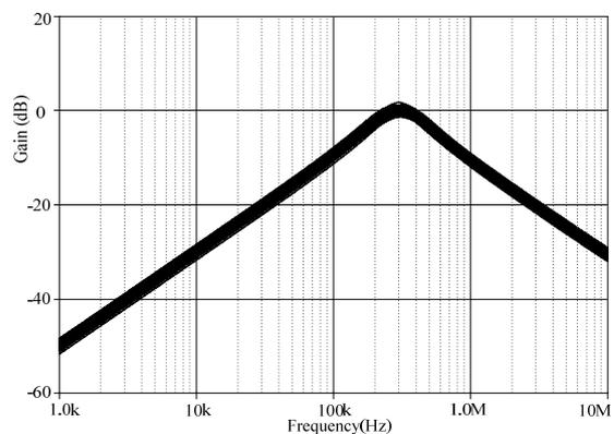
Fig.10. Simulated responses of bandpass for Monte Carlo Analysis
