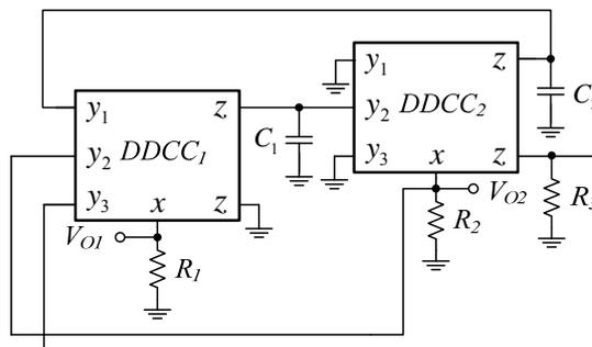
Fig. 3. Proposed quadrature oscillator
