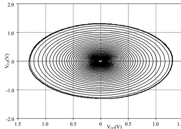
Fig.15. The Lissajous pattern of voltage output signals.
