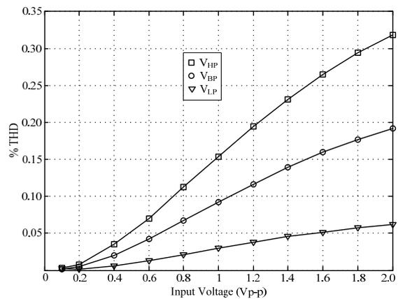
Fig.9. %THD for output voltage
