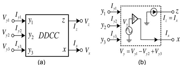
Fig. 1. DDCC (a) Symbol (b) Equivalent circuit
