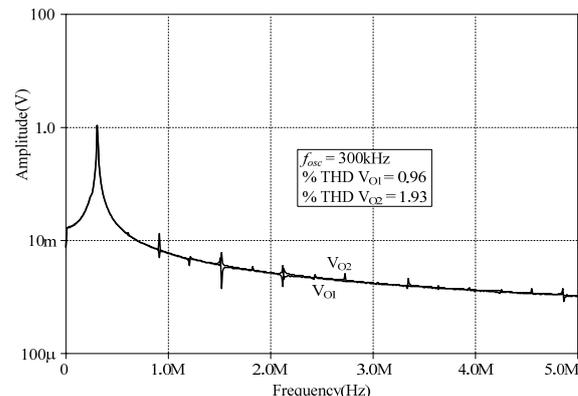
Fig.14. The frequency spectrum of output signals
