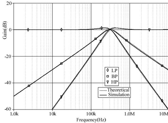
Fig.5. Frequency responses of voltage output
