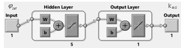
Fig.8. Structural diagram of the ANN reproducing the dependence  $k_{ac}(\varphi_{ref})$
