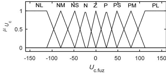
Fig.5. Membership functions of the output variable  $U_{c.fuz}$
