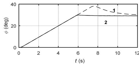
Fig. 3. Reaction  $\varphi(t)$  for a step control signal  $\varphi_{ref} = 30^\circ$ : 1 – without fuzzy corrector, 2 – with fuzzy corrector.
