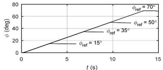
Fig.9. Reactions  $\varphi(t)$  of a plant's position with neuro-fuzzy corrector for reference step signals  $15^\circ, 35^\circ, 50^\circ$  and  $70^\circ$
