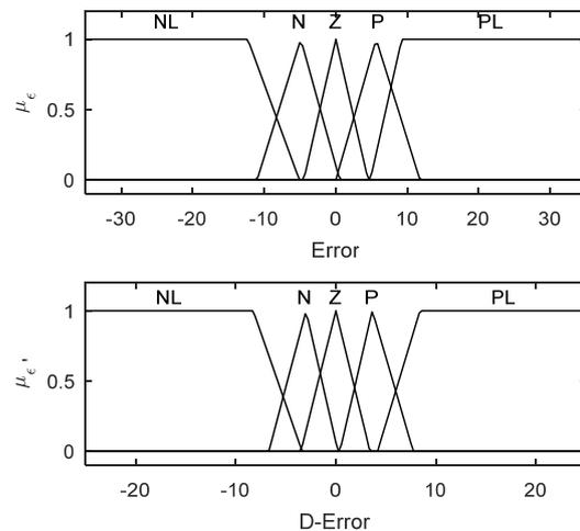
Fig. 4. Membership functions of the input variables Error and D-Error
