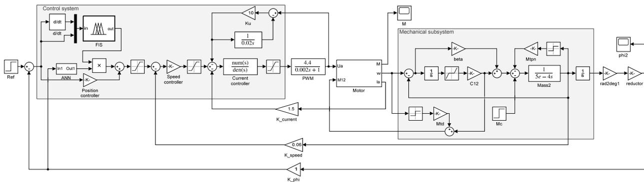
Fig. 1. Structure of the Simulink-model of the two-mass positioning EMS with triple-loop cascade control and with neuro-fuzzy corrector of proportional position controller: Ref—reference signal, ANN—artificial neural network, FIS—fuzzy inference system
