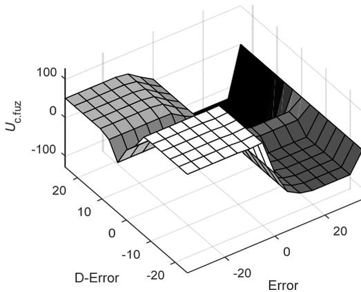
Fig.6. 3D surface of the designed fuzzy corrector FIS
