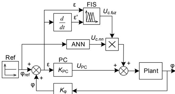
Fig. 2. Simplified functional block diagram of positioning electric drive with neuro-fuzzy corrector: Ref—reference signal, PC—position controller, ANN—artificial neural network
