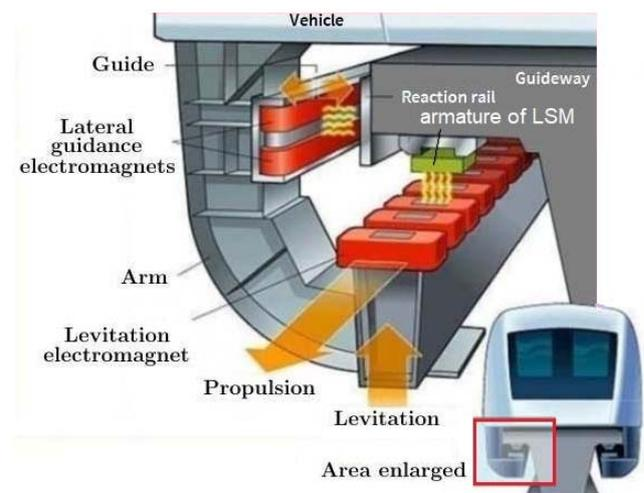
Fig. 3. Principle of operation of Transrapid maglev system.
