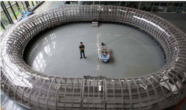
Fig. 12. Elliptical tube 45-m long built at State Key Laboratory and Traction Power, Southwest Jiaotong University, Chengdu, China for testing a small-scale magnetically levitated vehicle.
