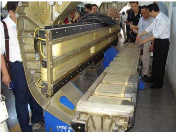
Fig. 6. Levitation (suspension) and lateral stabilization electromagnets. Five-phase winding of a linear generator is placed in pole shoes of levitation electromagnets.
