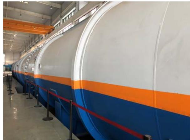
Fig. 14. Full-scale 140-m long evacuated tube at State Key Laboratory and Traction Power, Southwest Jiaotong University
