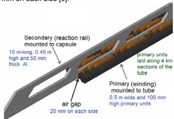
Fig. 10. Double-sided LIM for propulsion according to E. Musk [6]
