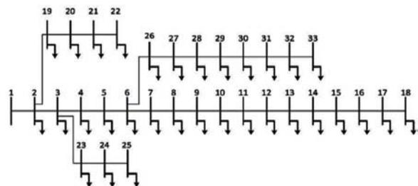
Fig.1. IEEE 33 bus test network
