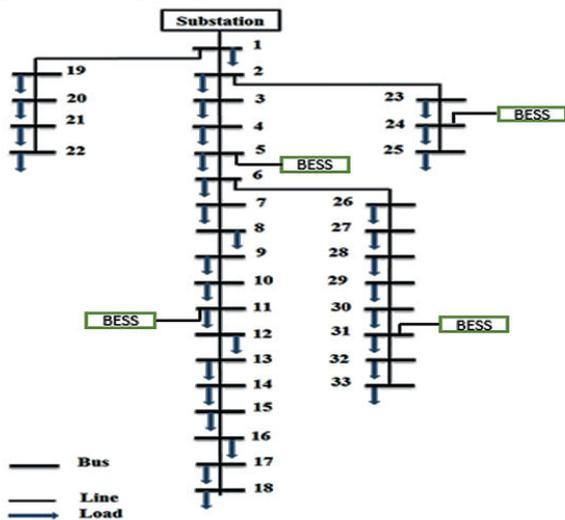
Fig.6. Optimal locations of Battery Energy Storage Systems
