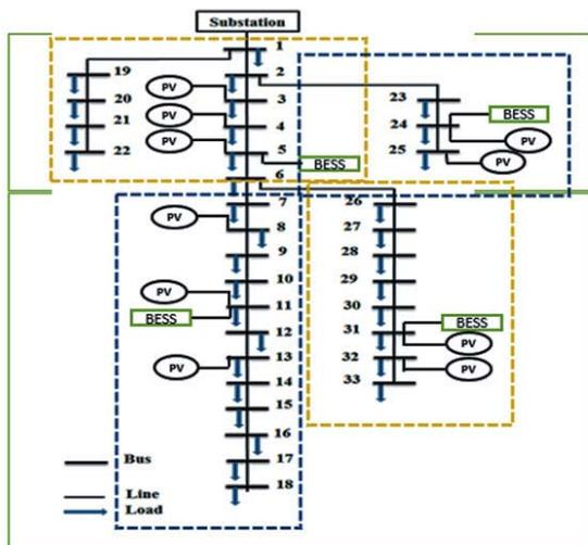
Fig.8. Optimal locations of photovoltaic systems and BESS-case 1
