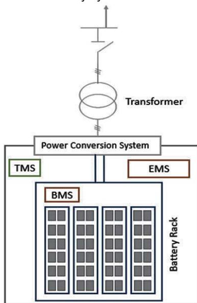
Fig.3. Elements of the Battery Energy Storage System
