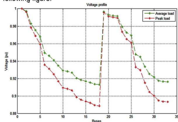
Fig.4. Voltage variation according to the number of buses
