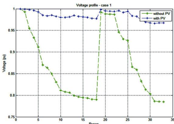
Fig.9. Voltage profile with and without integrated PVs-case 1
