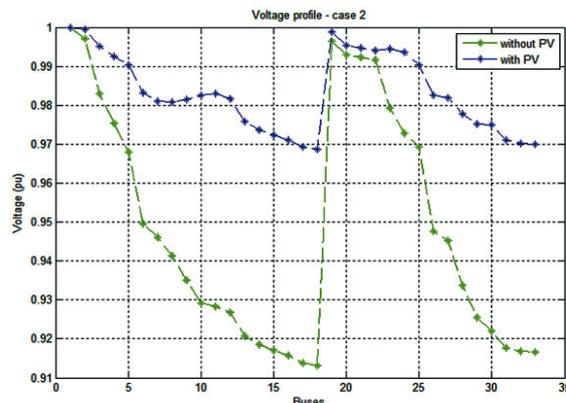
Fig.11. Voltage profile with and without integrated PVs-case 2
