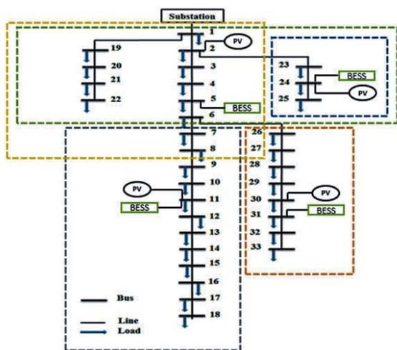
Fig.10. Optimal locations of photovoltaic systems and BESS-case 2
