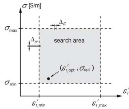
Fig.6. Limitations of the search area when determining the equivalent electric parameters
