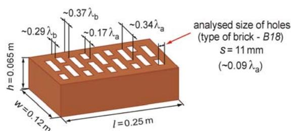
Fig.1. The electric and geometric sizes of the analysed brick
