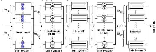
Fig. 8.1. Series- parallel power design
